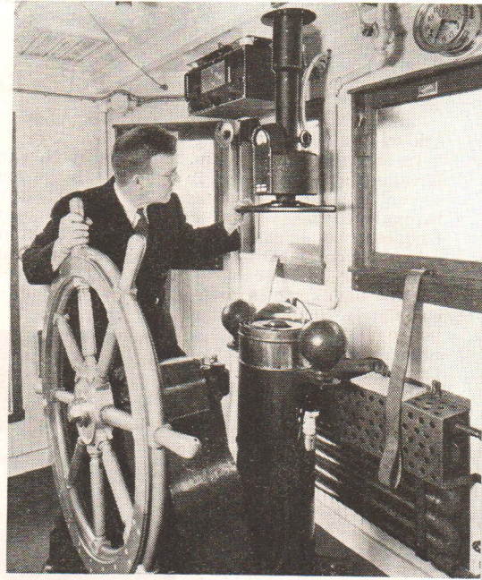
Marine compass installation. Operator has left hand on wheel which rotates the loop installed on the roof of the pilot house. (Photo Western Electric)
