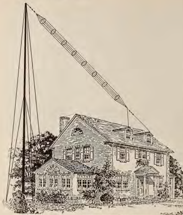
Fig. 5. Cage type of antenna popular with amateurs
