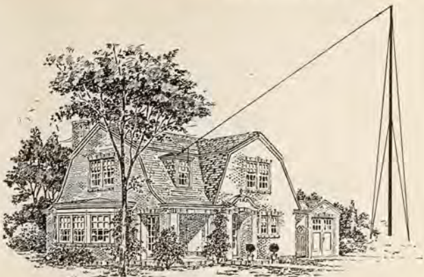
Fig. 4. Straight wire antenna for extreme simplicity
