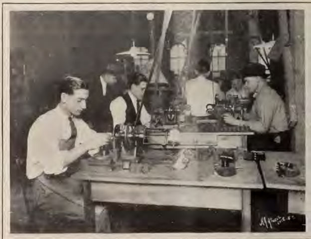
In the foreground is one of the machines used in winding primaries and interiors of torostyle coils. Finished primaries are seen under the spool of wire, while to the right are a few of the finished coils. Special machinery had to be developed for winding this type of coil, as explained in the article
