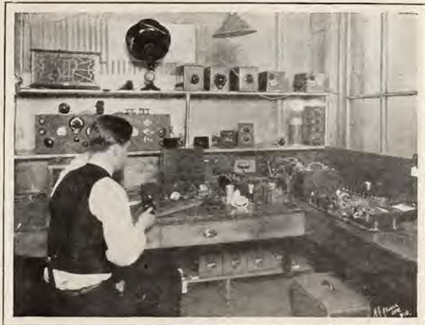
Here is a corner of the experimental laboratory where measurements on condensers and inductances are made. It is also here where preliminary tests are run on all apparatus before the company commits itself to the manufacture of a new article
