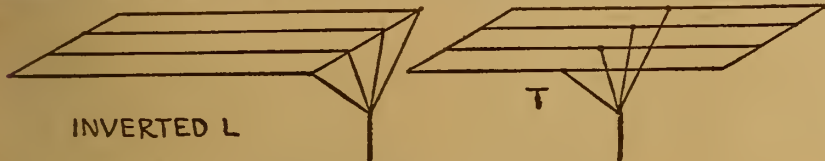
Figure 6—Two Types of Capacitive Aerials
