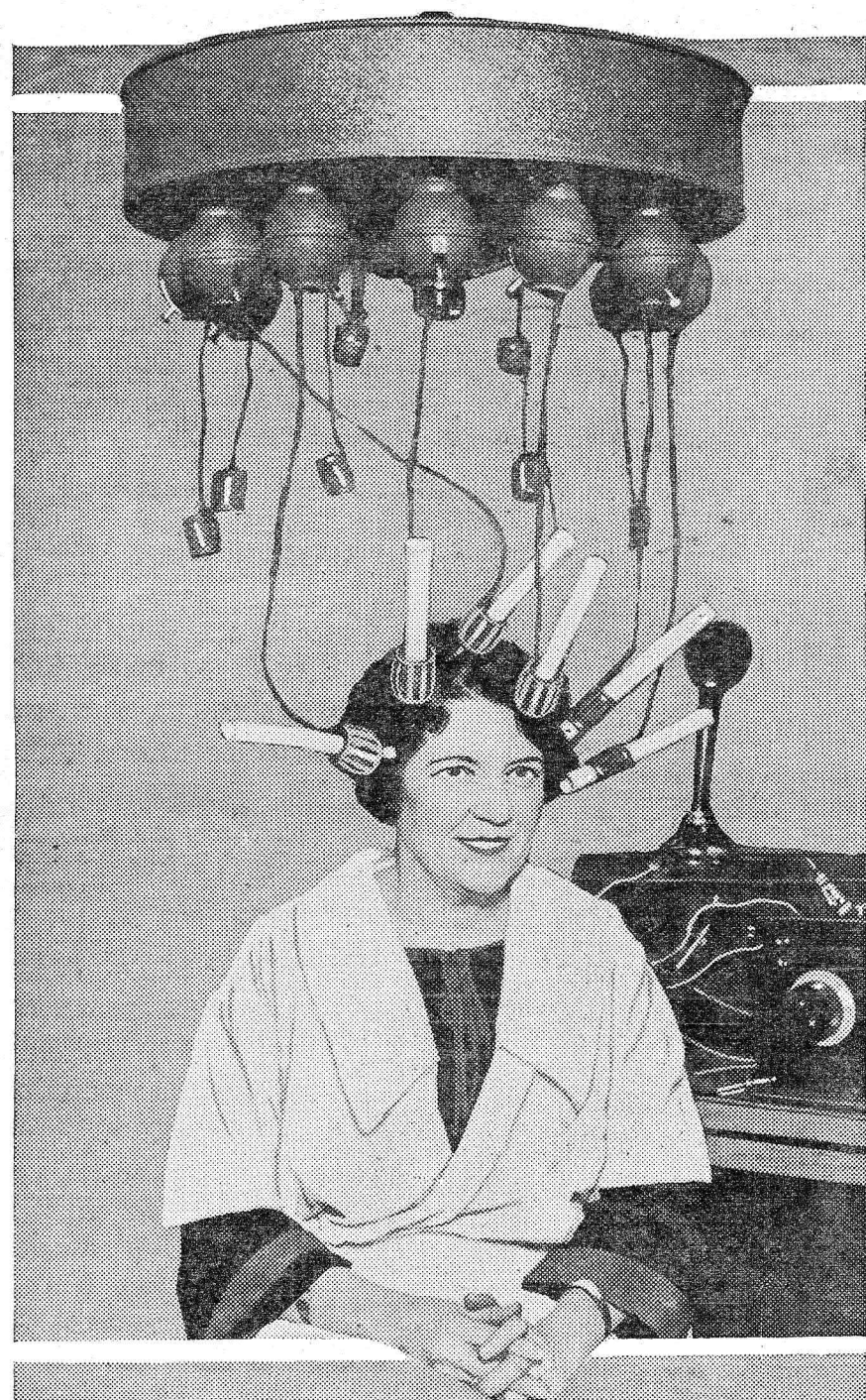
Milady can now have her hair waved by Radio. This machine produces a Radio frequency current of about 3800 meters wave length, it is claimed. The high frequency current is concentrated upon the subject's hair and used to produce heat. The current is circulated through strands of wire wound on a heating spool. The hair is wound for curling on a tube which is inserted into the spool. There is no heat until this tube is placed within the spool. The apparatus eliminates all possibilities of burning the subject or her hair, it is said. Int. Newsreel Photo
