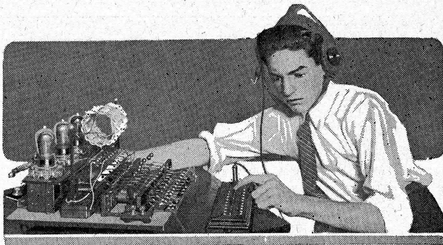
All one has to do to get a station is to press a button with that station's call letters upon it, and the machine pictured above automatically tunes in. The pressing of the button actuates electromagnets, which in turn cut in portions of the tuning coil. The set was displayed at several of the more recent Radio expositions.
