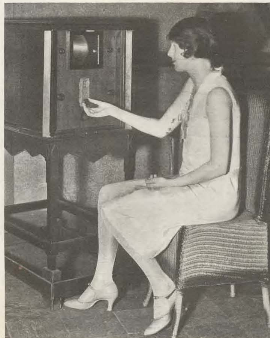
Television receiver. Picture is three inches square and has a pale, pinkish glow.
