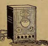
No more troublesome wire changing! Just connect the charger clips to the battery terminals and turn on the current-simple, quick and convenient. The France Super-Charger not only charges 120 volts of B battery in series but it also charges 2, 4, 6 or 8 volt A or Auto batteries, at a 5 to 7 ampere rate, tapering as the battery is charged.
