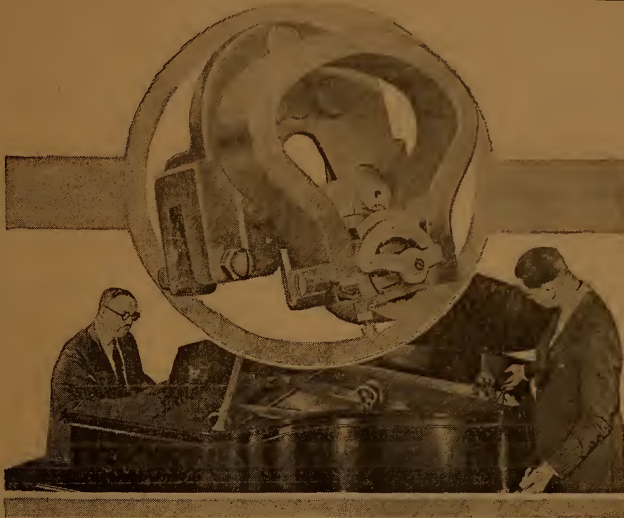
The remarkable instrument shown in the center insert is the new piano microphone developed and now used by the General Electric Company at their Schenectady station, WGY. Three of the devices are attached to the piano sounding board to pick up the high, middle and low notes respectively. The vibrations of the piano jar the floating armature of the three microphones, which are really miniature alternating current generators of special design. The jarring of the armatures makes electric currents that correspond in amplitude and frequency with the original piano tones. These electric currents are then superposed and used to modulate the high frequency carrier wave radiated by WGY. By individual control of each of the three "dynamo" microphones it is possible to blend the low, middle and high notes together so as to produce on the air an almost exact reproduction of the original piano sound
