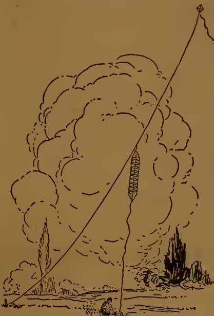
Figure 57—The spiral elevated by a kite for use with portable sets
