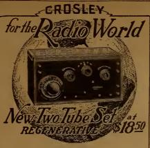
THE most astounding value ever offered in radio—a new two-tube receiver, Crosley Model 51, consisting of Armstrong regenerative detector and one stage of audio frequency Amplification. Licensed under Armstrong U.S. Patent No. 1,113,149.
