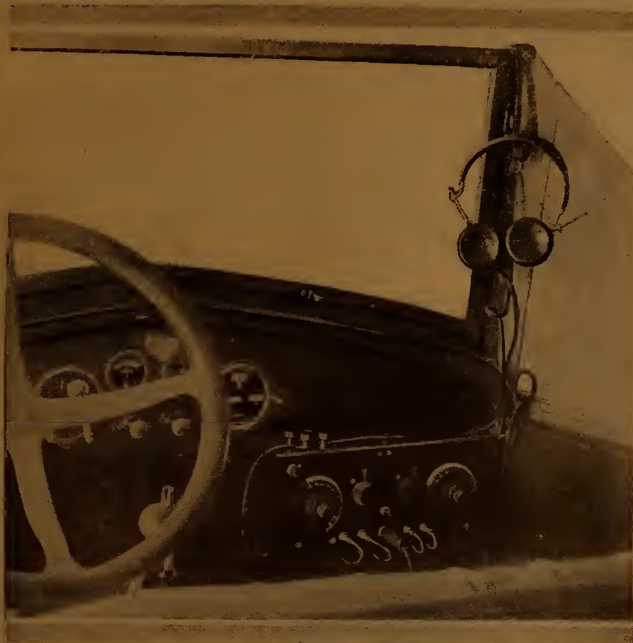
Showing installation of auto set below Essex dashboard.
