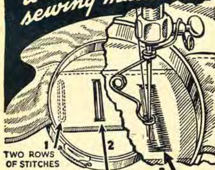
TWO ROWS OF STITCHES FOUR LONG STITCHES TO PAD BUTTON HOLE 3 SIDE-WAY FINISH STITCH
