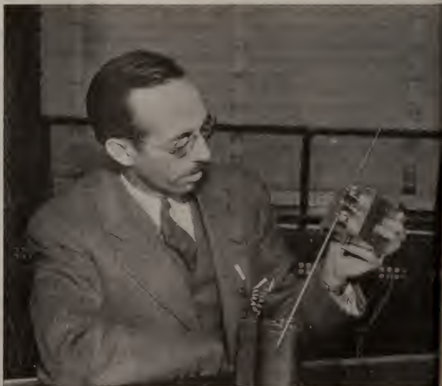
O. B. Hanson, Chief Engineer of the National Broadcasting Company, with the world's smallest Micro-wave transmitter, capable of flinging the human voice a distance of four miles. It operates on wave-lengths of one meter less at a power of .2-watt and was developed under Mr. Hanson's direction.
