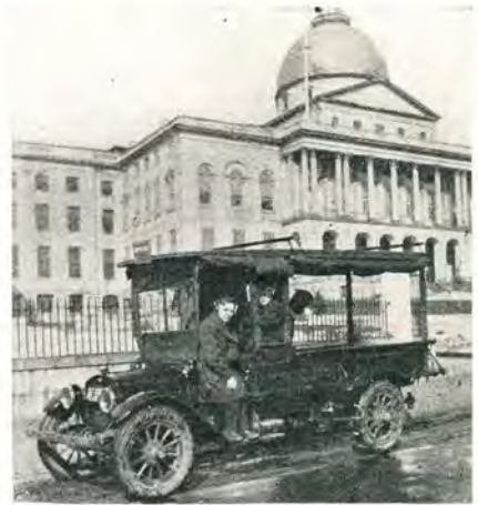
American Radio & Research Corporation truck equipped with receiver and 10-ft. aerial, with frame of truck acting as counterpoise, which picked up WDAP, WIP and other stations near Nantasket Beach, Mass.
