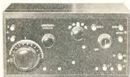
New model 51, made by Crosley, which has detector and one-stage of audio-frequency amplification. This is proving a very popular set.
