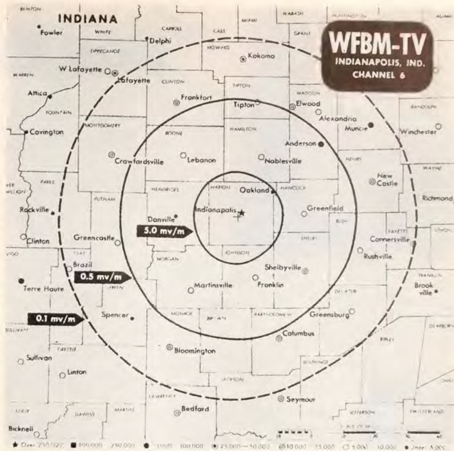
Millivolts per meter (mv/m) is measure of signal strength. Outer contour is over 50 miles out
