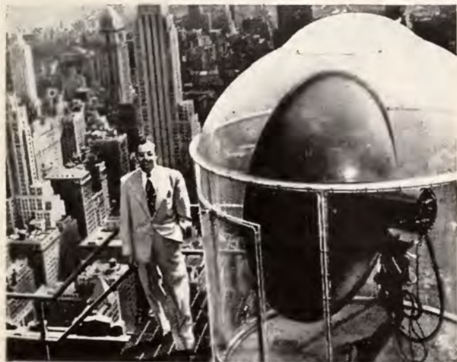
Bowl-shaped antennas at the parent television station pick up the microwave beam from the remote mobile van.
