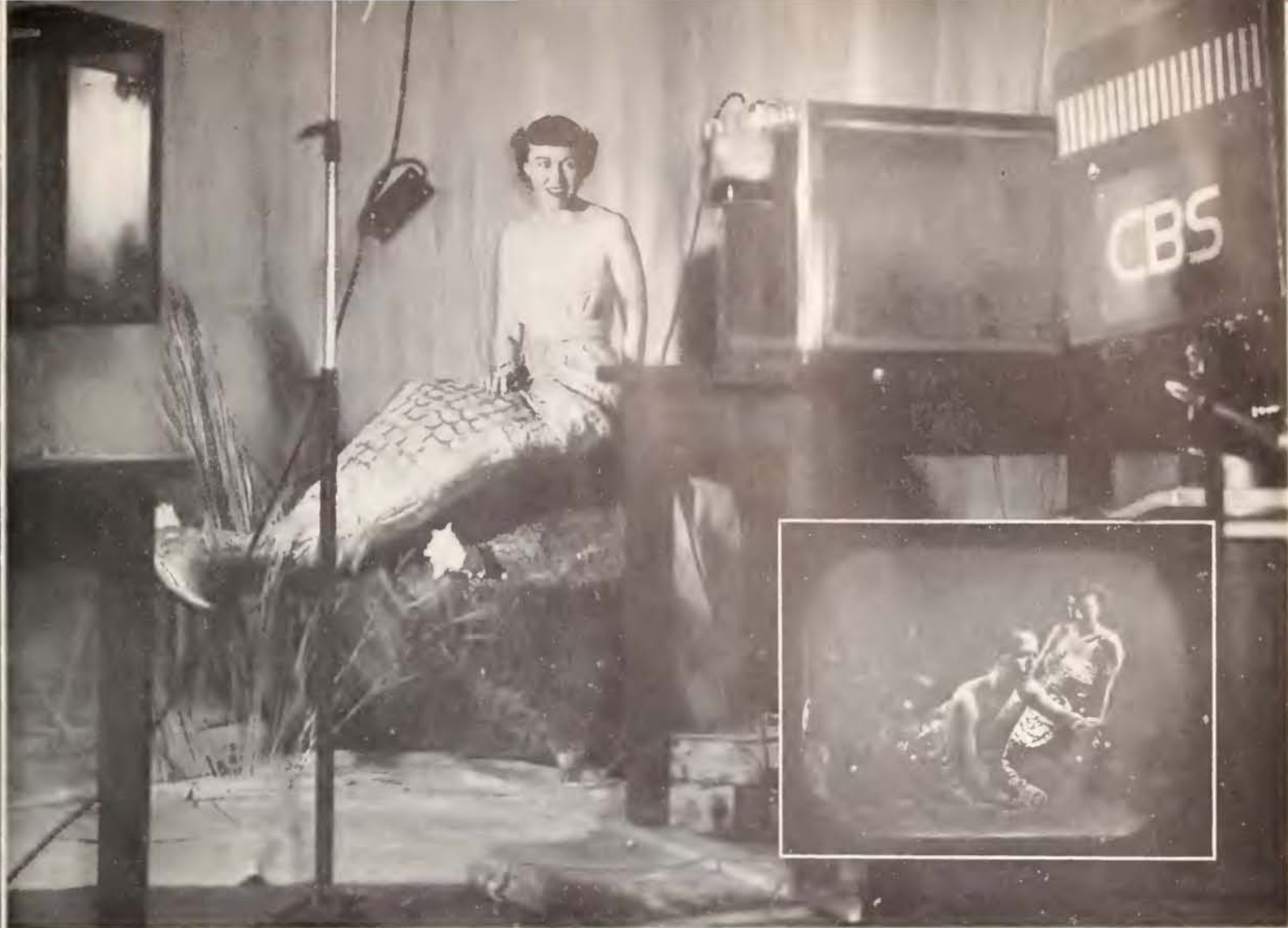
Superimposition: Illusion of underwater interview was created by the use of two cameras, one on CBS' Dorothy Doan, other on fish tank. See inset
