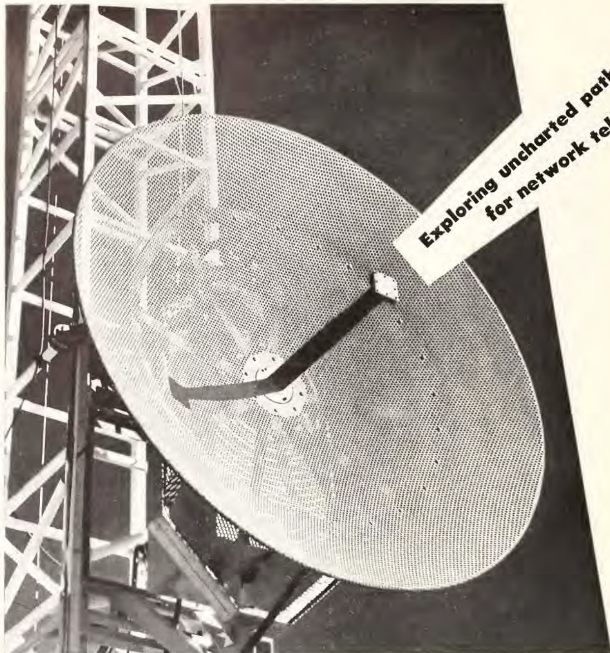
Portable microwave reflector—used in locating best radio relay routes
