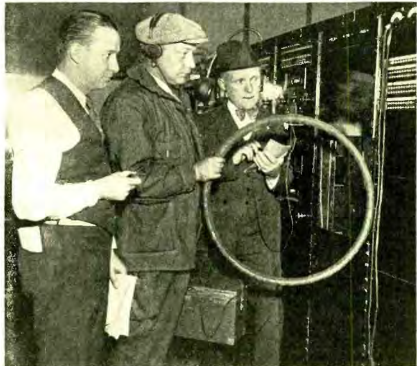
SLEUTHS Tommy Rowe, William Jackson and J. L. Riley, equipped with complicated apparatus, track down a mysterious buzzing in station broadcasts. Instruments located offending racket in a basement motor four blocks away.
