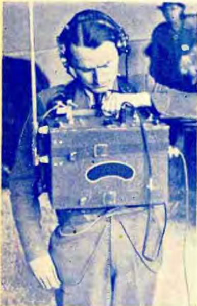
JIM DAUGHERTY carries considerable weight in the radio field when he sets out with the portable transceiver for use in remote broadcast pickups. It works on short waves.
