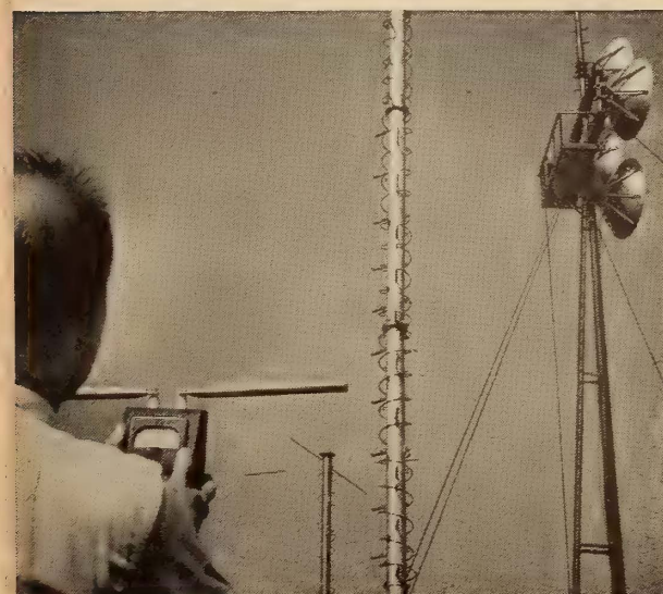
G-E HELICAL ANTENNA TEST. A field intensity test is run on a four-bay helical antenna installed at Electronics Park. The helical antenna, used with all UHF transmitters, boosts Effective Radiated Power up to 20-25 times.
