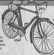
HERCULES ROYAL PRINCE LIGHTWEIGHT ENGLISH BICYCLE With Generator Powered Headlight
