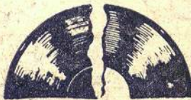
New Improved Record (Closer Grooved) Old Style Record (Grooved Too Far Apart)
