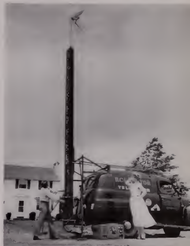
An RCA Service Co. truck which has an antenna which can be raised up to 70 feet, to test signal strength.
