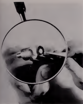
Magnified model of the two basic elements of the experimental RCA atomic battery, which by means of a new method makes it possible to convert atomic energy directly and simply into small but usable quantities of electrical energy.
