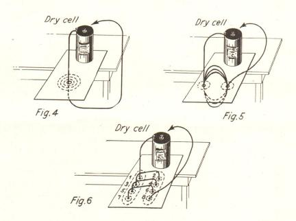
Theory of Action: When current flows through the wire, a magnetic field is built up around the wire. This field magnetizes the iron filings, causing them to take positions on the cardboard corresponding to the lines of force in the magnetic field.
