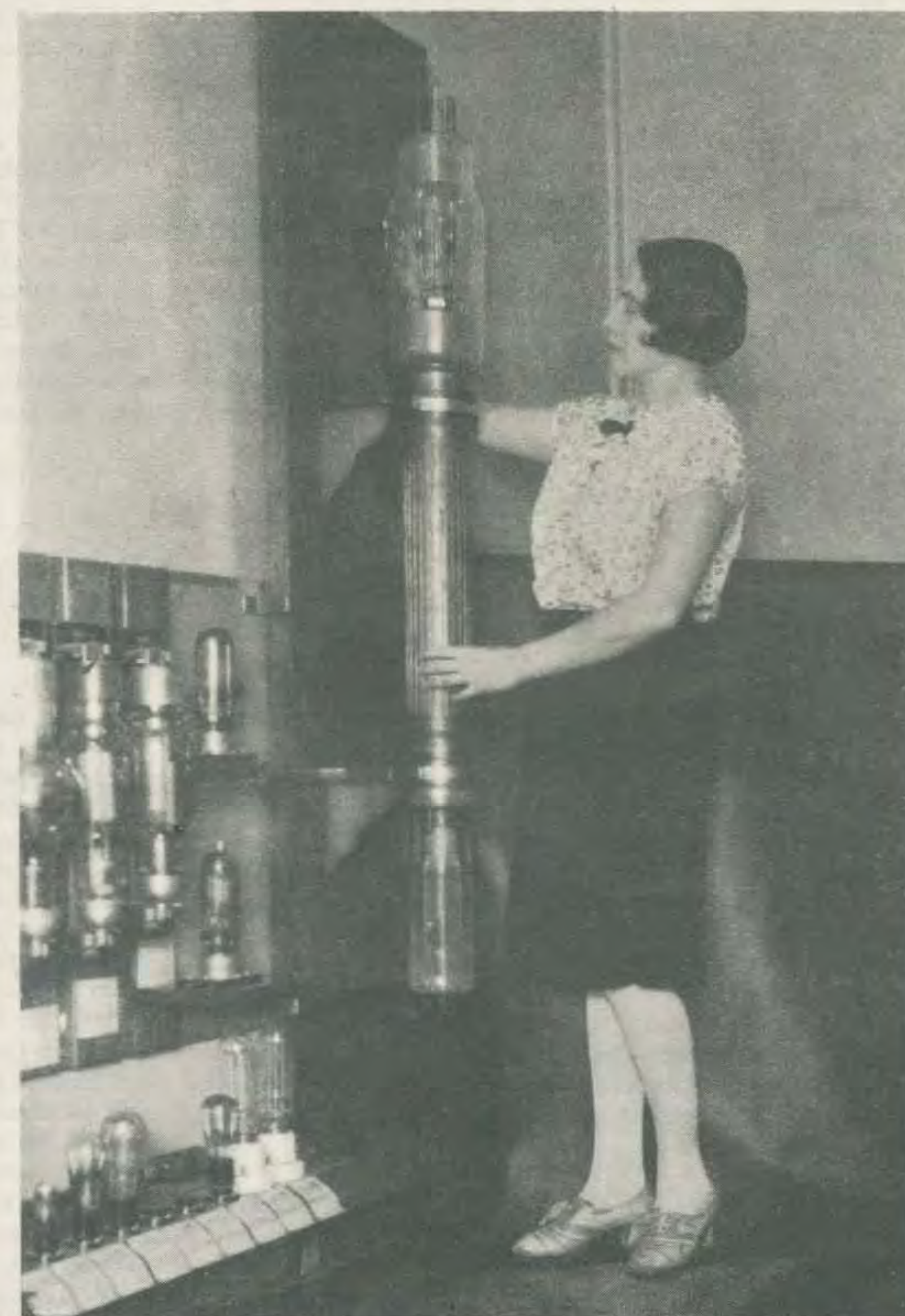
The new tube, designed by engineers of the Westinghouse Electric and Manufacturing Company, to be used in experiments with high power at the new KDKA station being erected at Saxonburg, Pa. This monster tube is six feet tall, weighs 60 pounds, and is cooled by five tons of water each hour of its operation!
