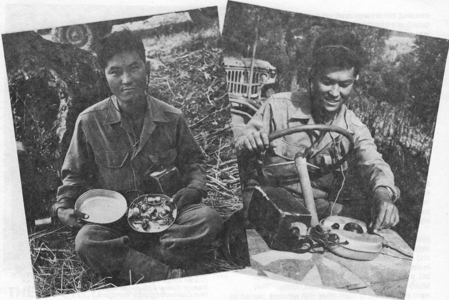
GI demonstrates, left, his combination mess kit and radio set and, right, attachment to his jeep, creating an "auto radio".
