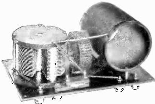
This is the interior of the crystal receiver previously described, and, as may be seen, the entire tuning equipment is mounted on a single Bakelite panel. A variable condenser is supplied for fine tuning and a lattice wound coil is used where wave lengths up to 2,500 meters are desired. This feature permits the reception of signals from the United States Government station at Arlington (Radio Va.)
