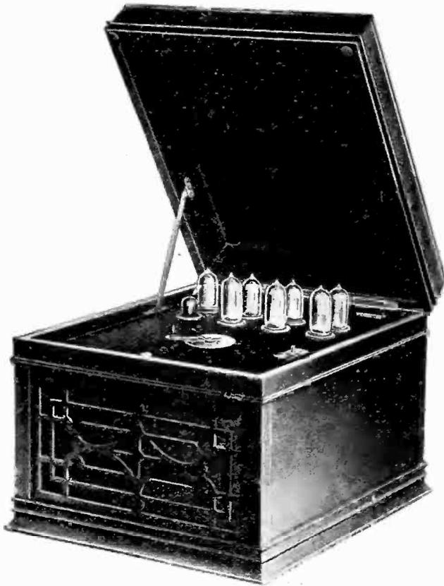
Aeriola Grand showing the vacuum tubes and ballast tubes in place, the switch which controls the entire current supply, and the single control lever used to tune in desired and tune out undesired broadcasting stations
