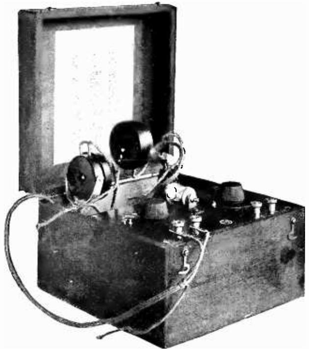
This is a complete crystal receiving set with two wave length controls, one of which acts as a fine adjustment on the other. This receiver is very useful for broadcasting reception. It may also be used to cover wave lengths up to 2,500 meters. It is marketed with a pair of sensitive telephone receivers
