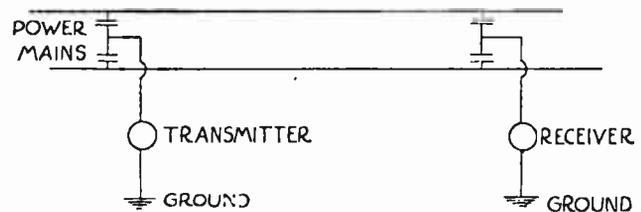
mains. For the radio currents the two mains are connected in parallel and used as one conductor, the ground being the return conductor. Good results are also obtained by connecting the transmitters and receivers between the mains, suitably protected by condensers to keep the large power current from passing through the radio apparatus, but the arrangement indicated above is more suitable.
