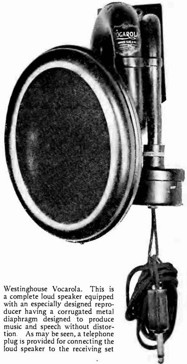
Westinghouse Vocarola. This is a complete loud speaker equipped with an especially designed reproducer having a corrugated metal diaphragm designed to produce music and speech without distortion. As may be seen, a telephone plug is provided for connecting the loud speaker to the receiving set
