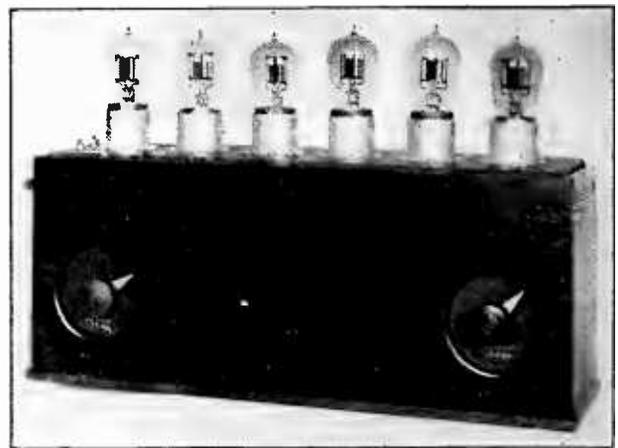
Exterior view of a new amplifying unit made by the Wireless Specialty Company for its use in conjunction with loop aeri- als and loud speaker. Six vacuum tubes are employed, but they function as eight, because two of the tubes are used twice. The complete unit operates as five stages of radio frequency, detector, and two stages of audio frequency. This unit has been built more for demonstration purposes than for general use.
