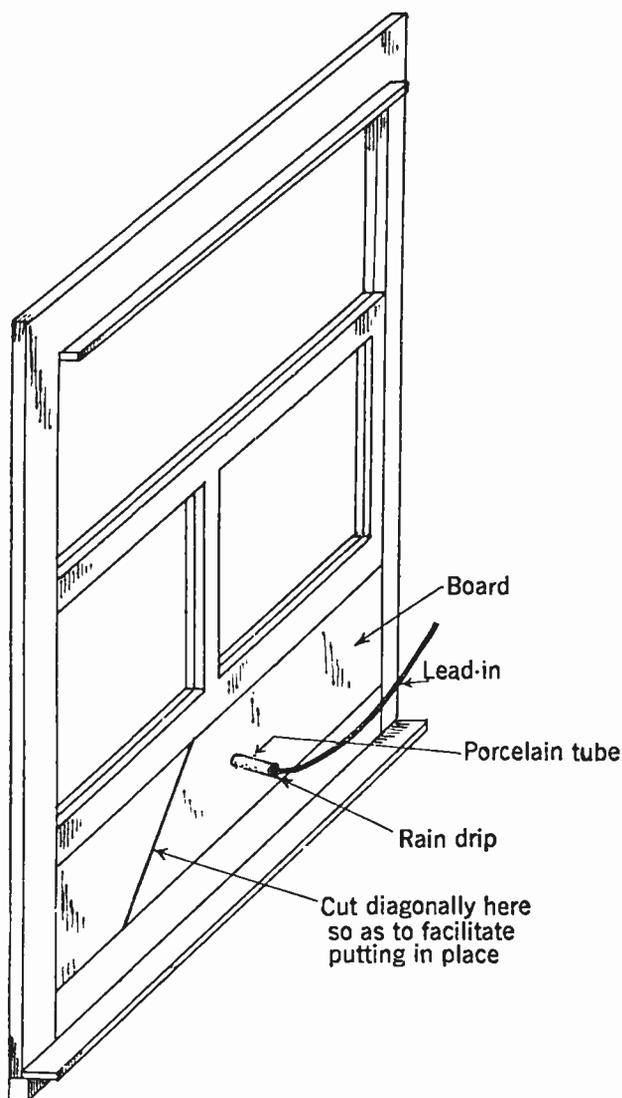
Fig. 11. Method of bringing lead-in into house
