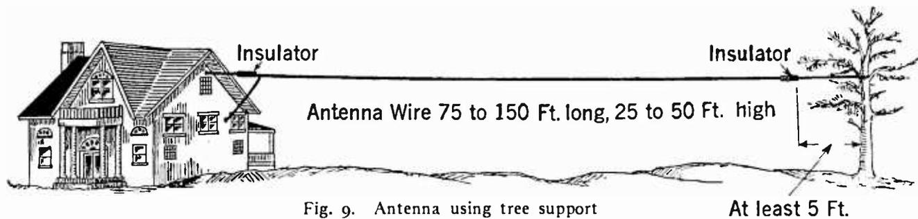
Fig. 9. Antenna using tree support
