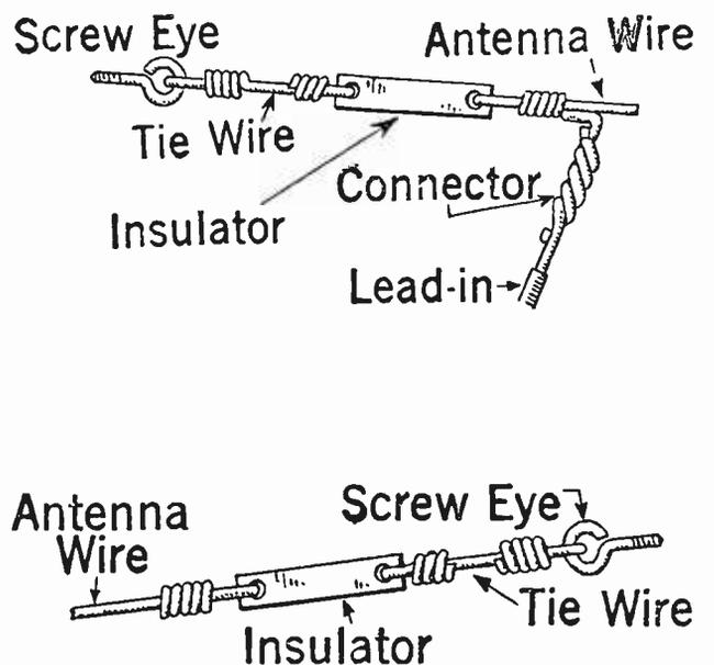
Fig. 6. Details of antenna construction
