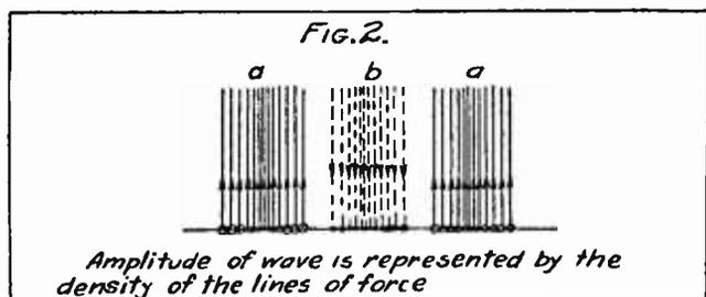
figure shows a radio wave moving from left to right. The electrostatic lines of force are represented by lines, the magnetic lines of force are represented by little circles at the end of the lines. It must be remembered that these are lines though they cannot be shown as such in a simple drawing. They extend at right angles to the electrostatic lines of force. In other words they extend away from you and into the paper as you look at the figure.
