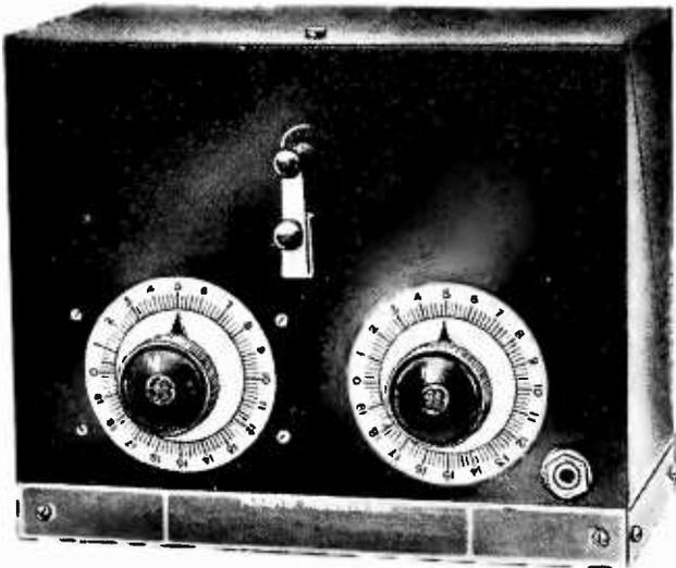
Exterior new General Electric short wave tuner embodying many new features. This tuner may be used with a crystal detector or vacuum tubes. An important feature is the metal case, used instead of the usual wood cabinet. This metal furnishes an effective "shield," preventing capacity effects between the receiver itself and the body of the operator
