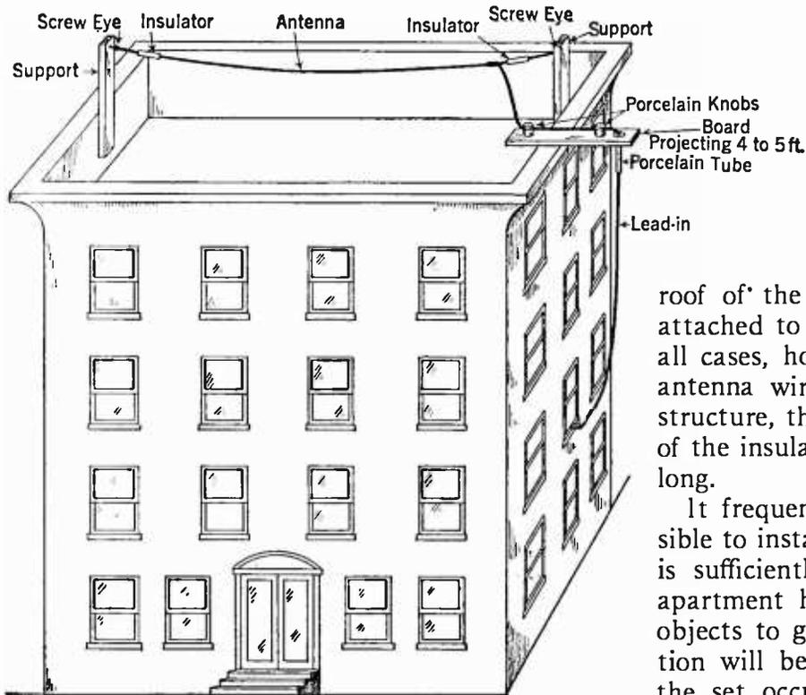
Fig. 7. ANTENNA ERECTED ON APARTMENT
