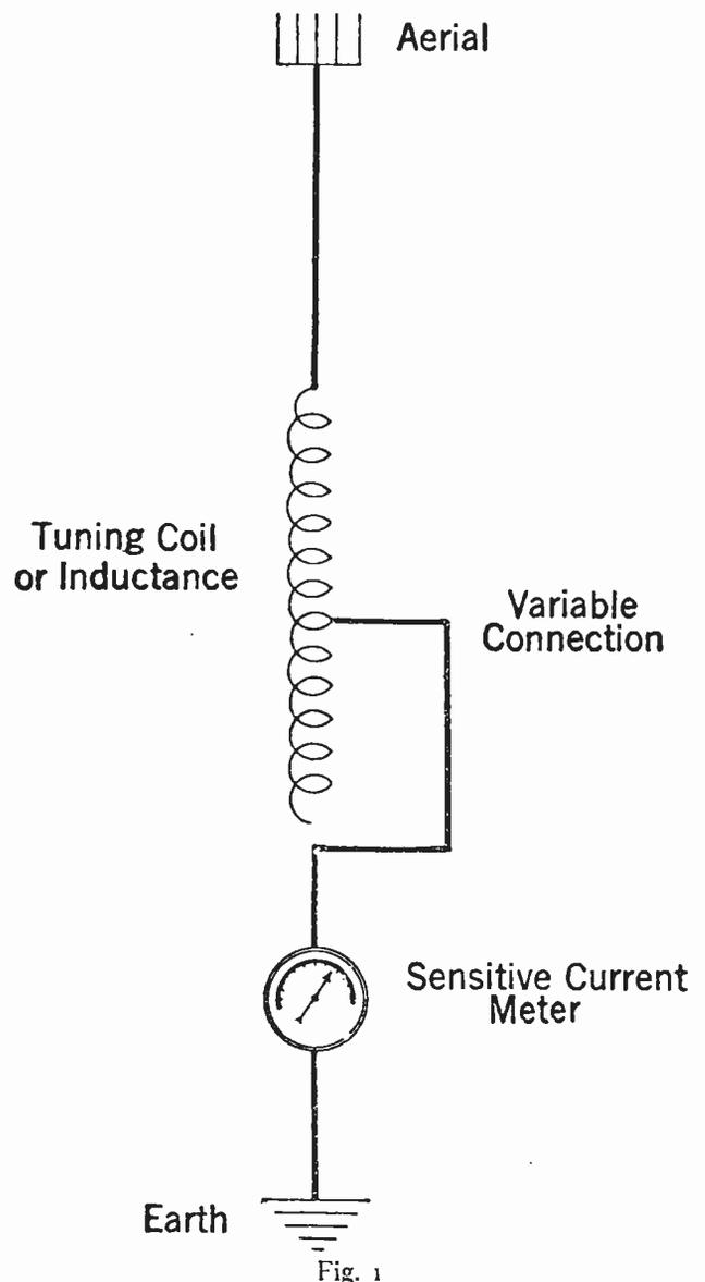
electric currents flowing in the aerial-to-ground circuit. These currents will alternately flow up and down, the frequency of complete (double) reversal being identical with the frequency of the arriving radio wave. The currents will last as long as the radio waves continue to strike the aerial; when the wave ceases, the currents will rapidly die away.
