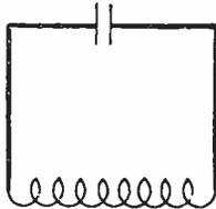
Fig. 1. An oscillatory circuit
