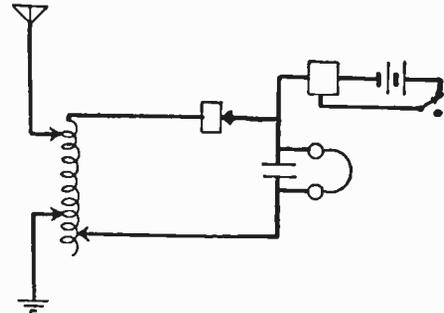
Fig. 4. Crystal receiver circuit showing test buzzer connections
