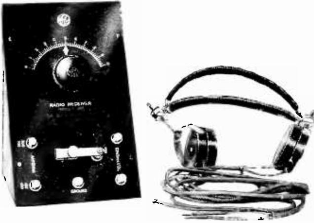
This is a new General Electric crystal receiving set complete with telephone receivers now being featured by the Radio Corporation of America. This little receiver has a wave length range of 180 to 700 meters, made in two steps 180 to 400 and 300 to 700 meters respectively, and tuning is accomplished by a single control to which a pointer is attached which moves over a graduated scale. When the set is not in use, the receivers may be placed inside the metal case by removing the front
