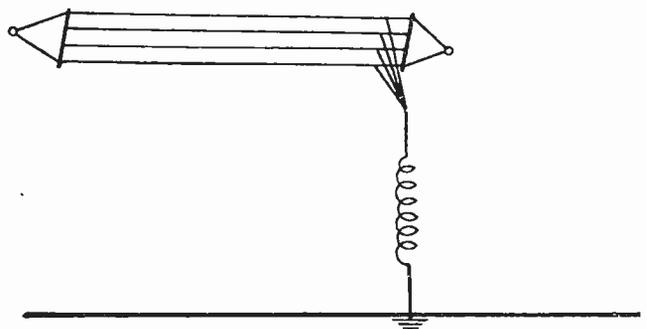
Fig. 2. The antenna circuit as an oscillatory circuit
