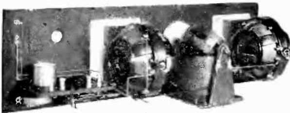
This is the interior of the 150 to 1,000 meter receiver, and, as may be seen, the vario coupler and variometers are of new design and are entirely shielded to prevent body capacity effects
