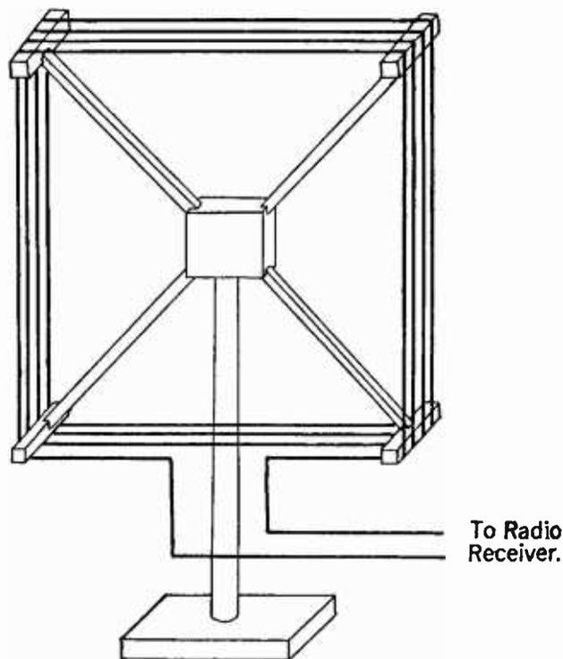
Fig. 10. Loop antenna
