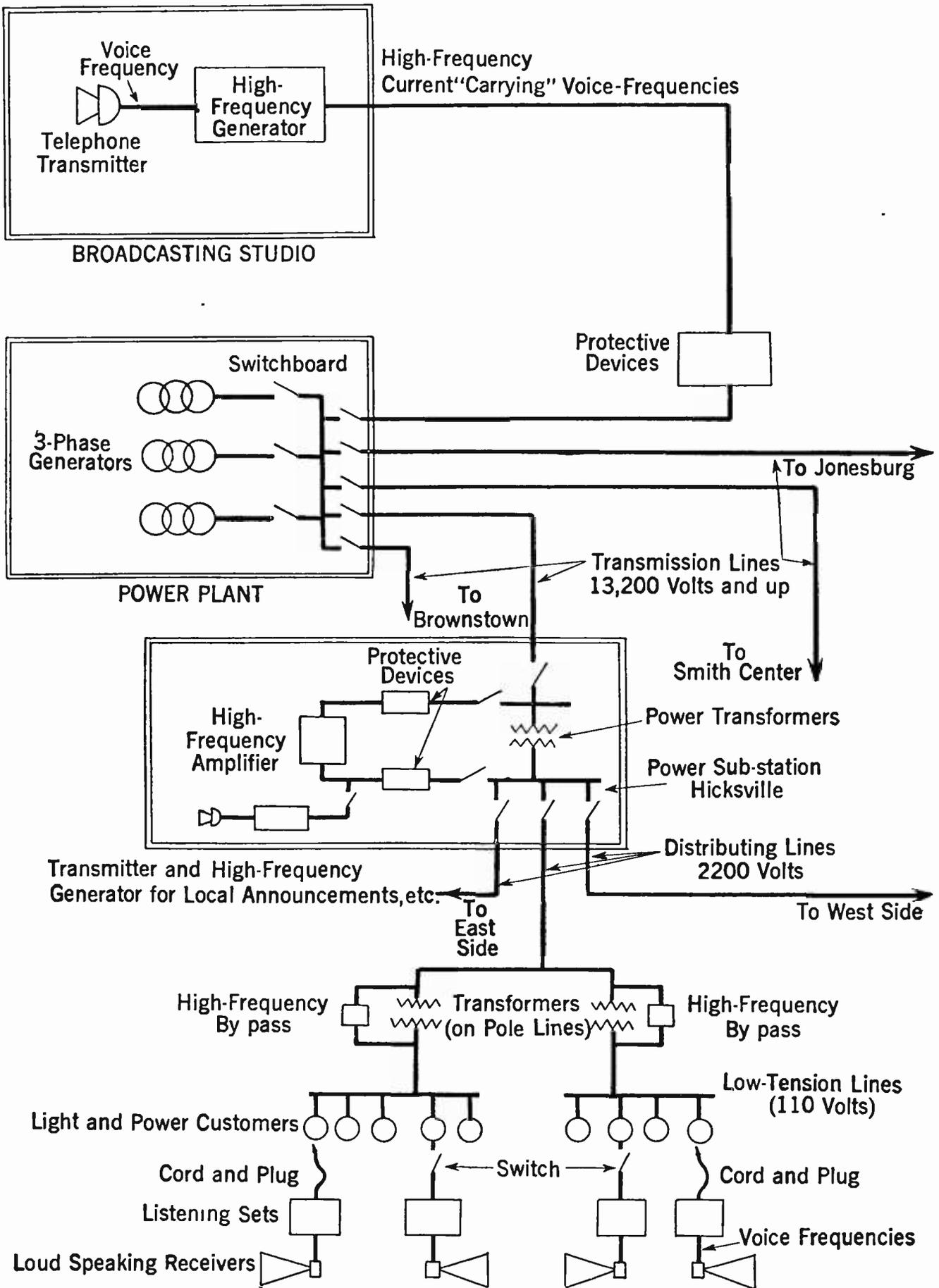
Fig. 1. Diagram of Carrier Broadcasting Set-up.
