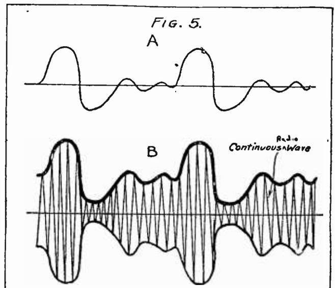
wave similar in character to that of figure 4. It has been found possible to do this by varying the amplitude of the radio waves so that this variation in amplitude follows in detail the wave variation produced by the sound. In figure 5, curve A represents a simple sound wave.
