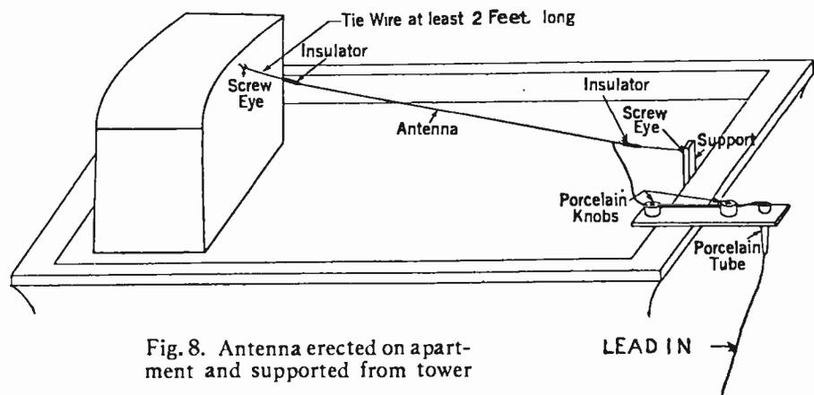
Fig. 8. Antenna erected on apartment and supported from tower
