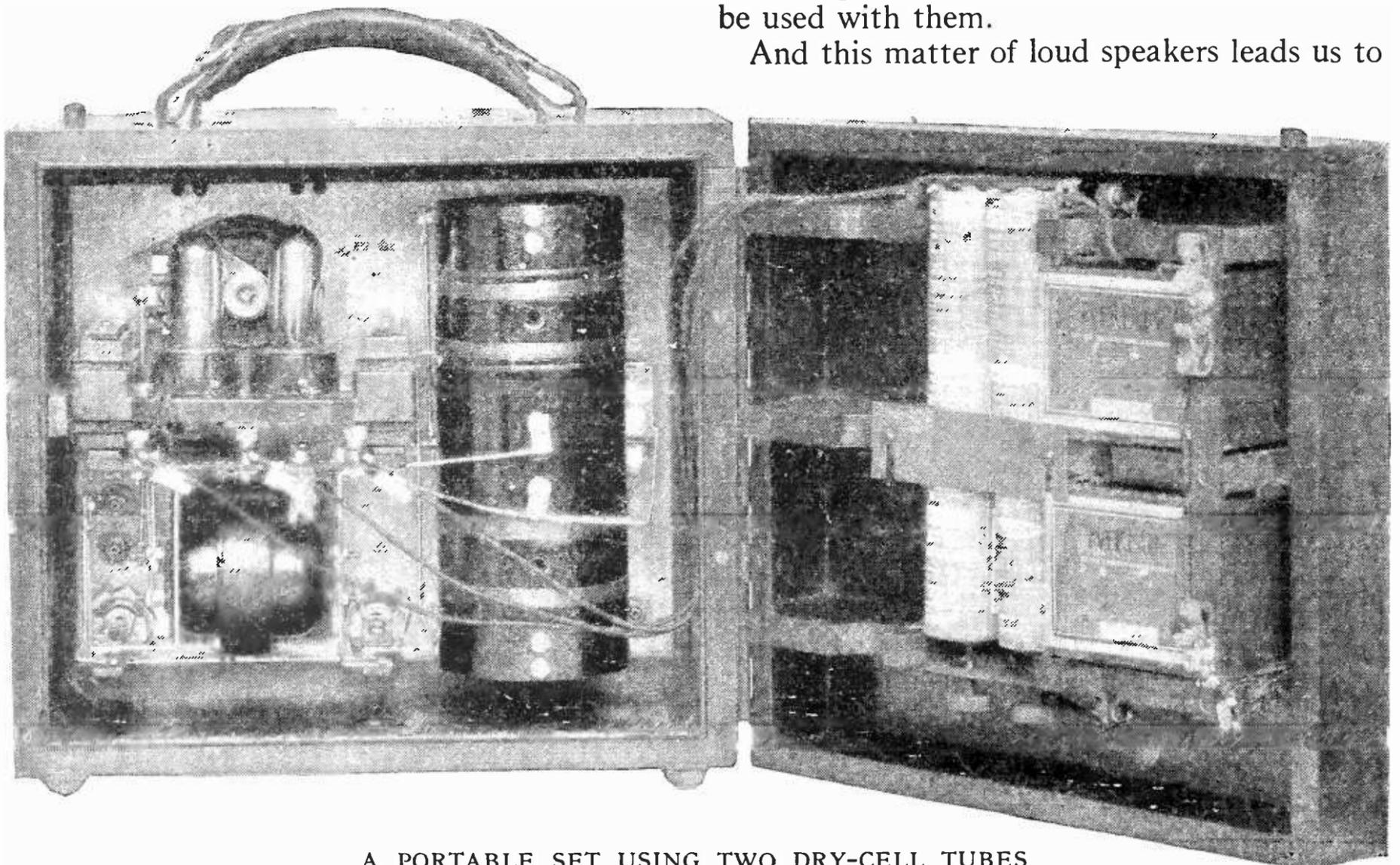
A PORTABLE SET USING TWO DRY-CELL TUBES
