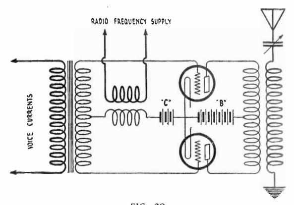
FIG. 20 A "balanced modulator" system which eliminates the carrier wave
