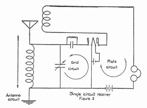
regeneration is apparently a method of decreasing resistance to a very low value, which permits large currents to flow. Another important result is the increase in selectivity also due to the lowered effective resistance.
