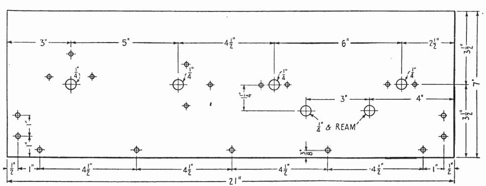
FIG. 5 The panel layout for the Four-Tube Knock-Out
