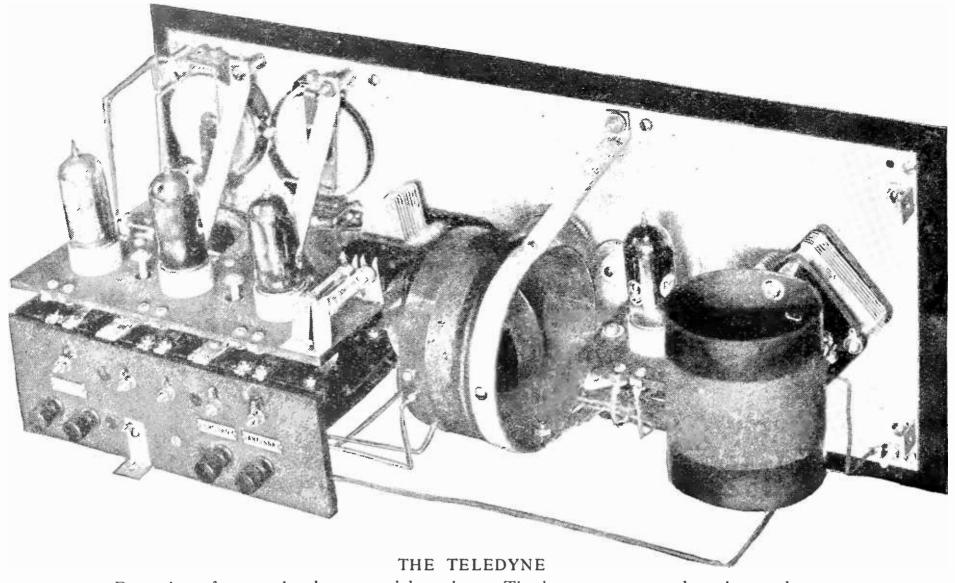
Rear view of a completed commercial receiver. The home constructor by using good parts which he may select himself and mount on a panel as suits him best, can easily build this set
