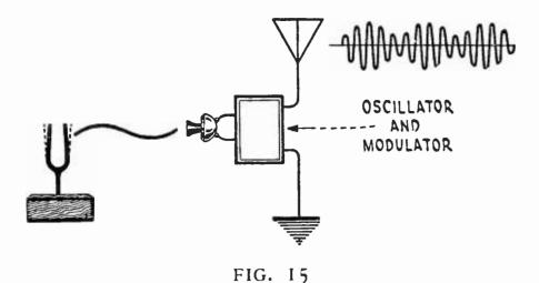
A continuous radio wave modulated by an audio-frequency impulse from the tuning fork
