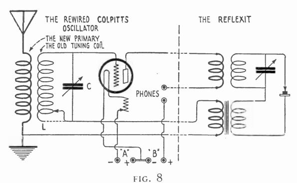
The complete circuit—the re-wired blooper plus the Reflexit. This is a real receiver
