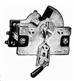
ing it unnecessary to use shielding. The vernier control used makes extremely fine tuning possible as well as accurate logging. Made by Hammarlund Mfg. Co., Inc.,
