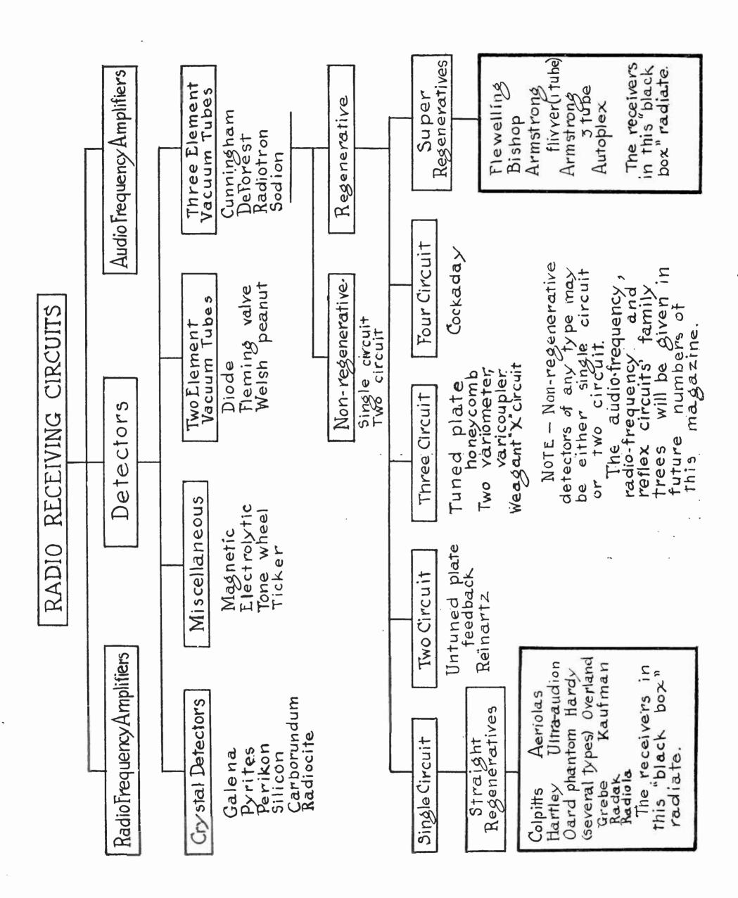
radio-frequency circuits: the antenna and ground, the secondary or input of the detecting device, and the output. If the output is not tuned, that is, if there is no attempt to resonate it with the radio-frequency signals, the system becomes a two-circuit tuner. If the antenna to ground circuit is combined with the input, the combination is known as a "single circuit" receiver.
