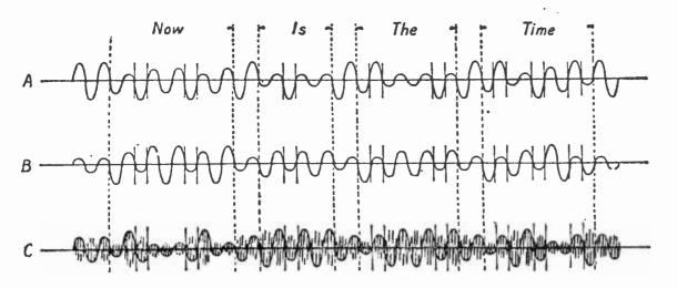
(A) Dot—smallest amplitude. Dash—medium amplitude. Space—largest amplitude.
