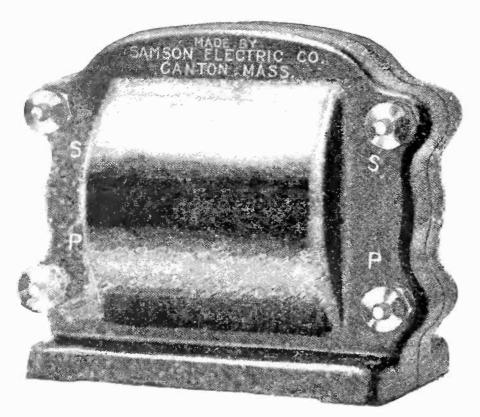
Samson Audio Transformer. A rugged transformer employing the helical winding, which avoids the necessity for paper insulation between layers, thus reducing the capacitance effect. Made by Samson Electric Company, Canton, Mass. Price \$7.00
