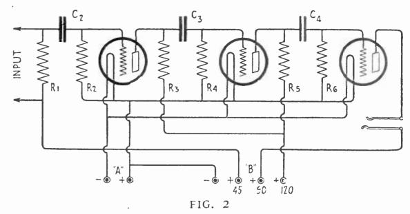
The fundamental circuit of a three stage resistance-coupled amplifier
