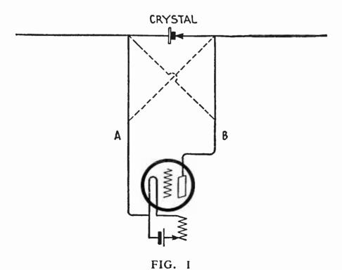
The principle which may be followed in substituting a two element valve for the crystal detector in any circuit
