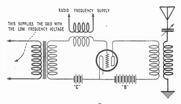
FIG. 18 A simple method of modulating a vacuum tube
