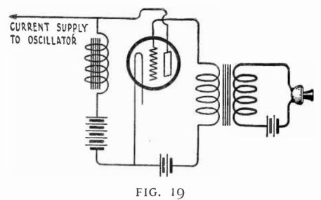
A commoner method of vacuum tube modulation
