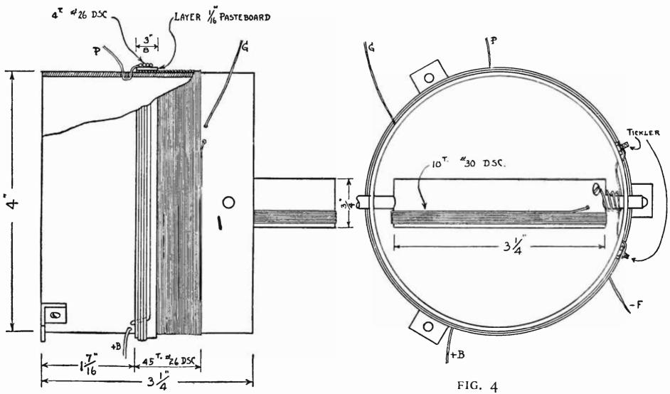
Detector grid coil, R. F. plate coil and regeneration coil
