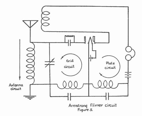
one of obtaining resonance or of conveying energy from one circuit to another. For instance the "X" circuit in which the plate is tuned with a fixed coil in series with a variable condenser in place of the usual variometer is still a tuned plate arrangement.
