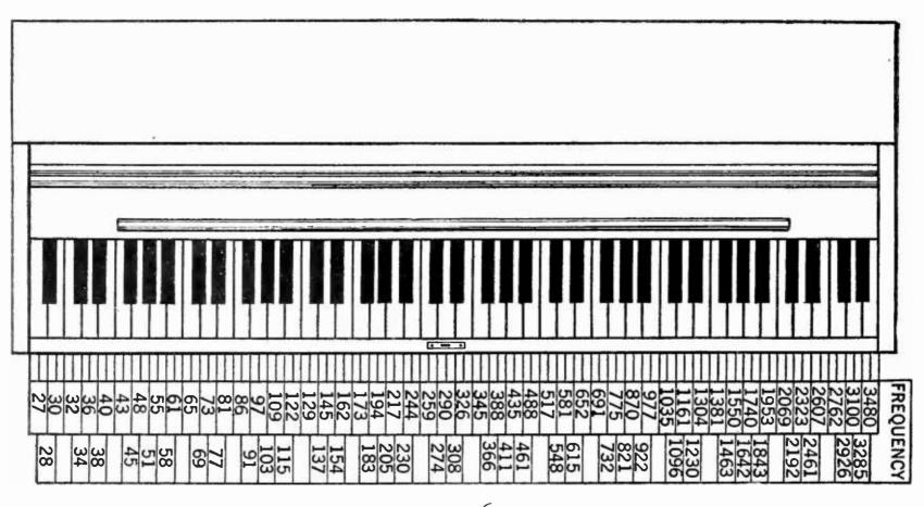
FIG. 6The frequencies and corresponding wavelengths of the sounds produced by the keys on a piano
