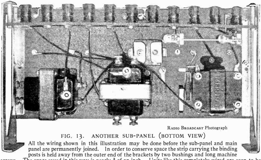
screws. The space saved in this way is nearly  $\frac{3}{4}$  of an inch. Units like this completely wired are soon to be placed on the market. The Radio Research Laboratories, New York City, are the originators of this unit idea. It would be well to compare this illustration with Fig. 7 to note the changes
