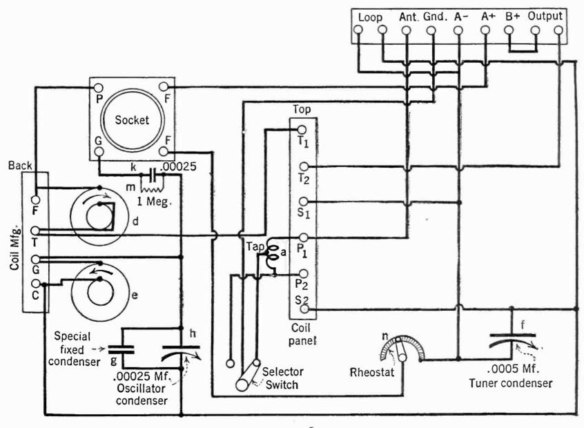
FIG. 6The wiring diagram of the one tube super-heterodyne showing the connections of the various units
