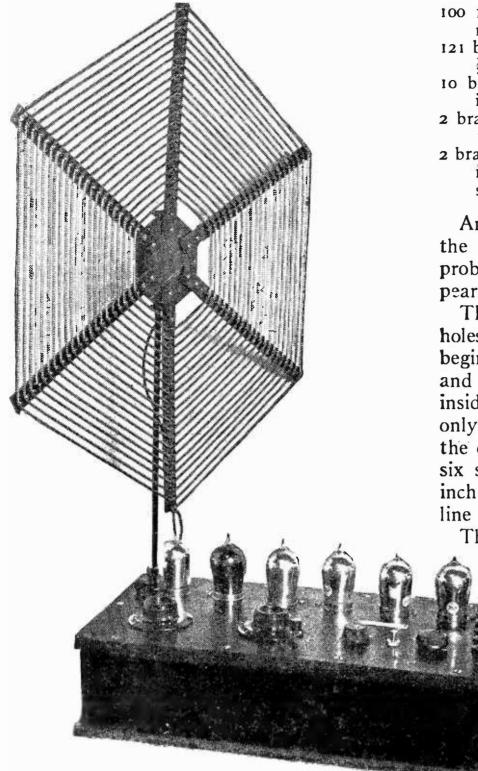
RADIO BROADCAST Photograph FIG. 9 An attractive and efficient coil antenna
