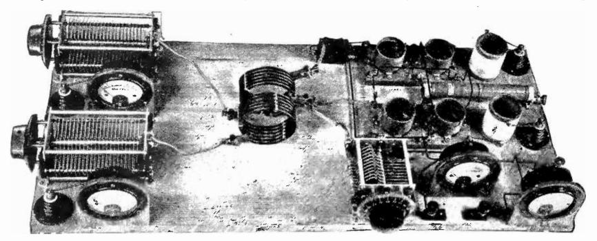
THE 200 WATT TUBE TRANSMITTER For use on very short waves which Mr. Schnell will use for experimental communication while he accompanies the Navy fleet on its Pacific cruise this summer
