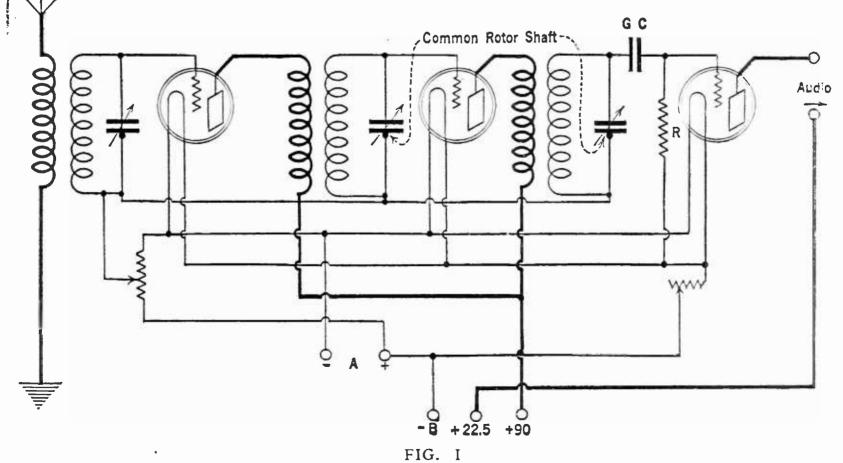
Simultaneous tuning of the conventional r. f. circuit. Note the grid condenser-grid leak connections
