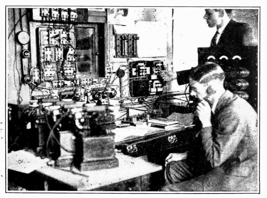
APPARATUS AT THE GLASGOW STATION Of the British Broadcasting Company. Many of the switches in the foreground are for controlling the wire lines between the various stations
