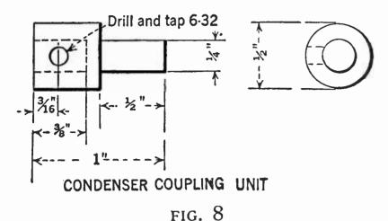
To shield the condenser from body capacity effects it should be placed some distance from the panel and this coupling member enables the proper spacing to be carried out
