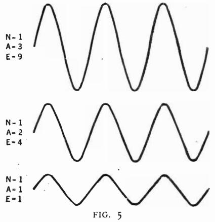
Waves of similar frequency, but of differing amplitudes. This drawing shows that the energy of a simple wave is proportional to the square of the amplitude, the frequency remaining constant
