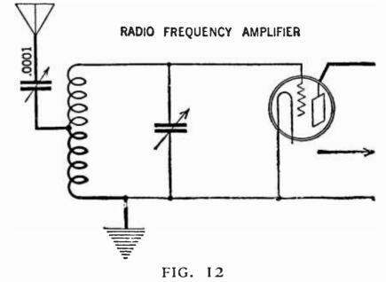
A simple method of increasing selectivity is illustrated in this Figure. The condenser may be variable, but after the correct place to tap the coil is found there is no need for further adjustment
