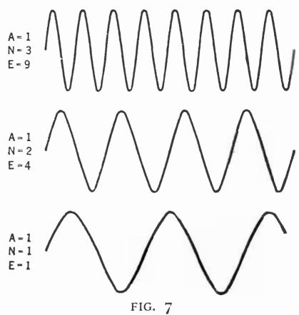
Waves of the same amplitude, but of differing frequency. The energy is shown here as proportional to the square of the frequency when the amplitude is the same
