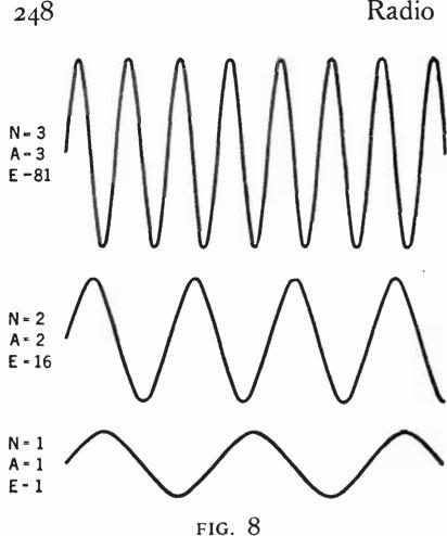
Waves whose frequency and amplitude are both different. The energy is here shown as proportional to the product of the amplitude squared and the frequency squared
