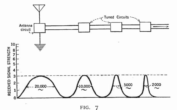
A coil and a condenser are the requisites of an obstacle to put in the path of a radio frequency current. Such a device, if properly used, may sharpen the tuning because it must be accurately tuned before any energy can get through. Two or more increase the selectivity because nothing gets through until each obstacle is tuned correctly
