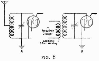
It sometimes happens that the antenna is connected to the receiver as shown in A of this Figure and the method of adding the Frequency-Changer is illustrated in B, where a few turns of wire are wound around the grid coil of the first tube
