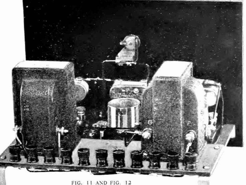
The top side with all parts excepting the bypass condenser in view. Note how the two audio transformers are mounted with their cores at right angles to each other. Much of the wiring is on the under side of the sub-base the transformer in place, mark the holes with a scriber.
