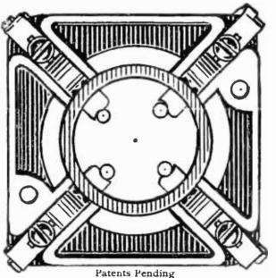
Interior view from bottom showing new method of direct connected side-contact, elastic, phosphor-bronze spring assembly. (Universal details not illustrated)
