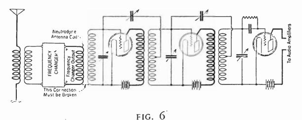
The addition of the Frequency-Changer to a receiver like that of Fig. 5 is a simple matter as this diagram shows. It is important that the connection indicated be broken to avoid shorting the B battery
