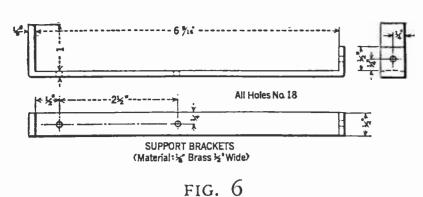
The angle bracket details. Two are required
