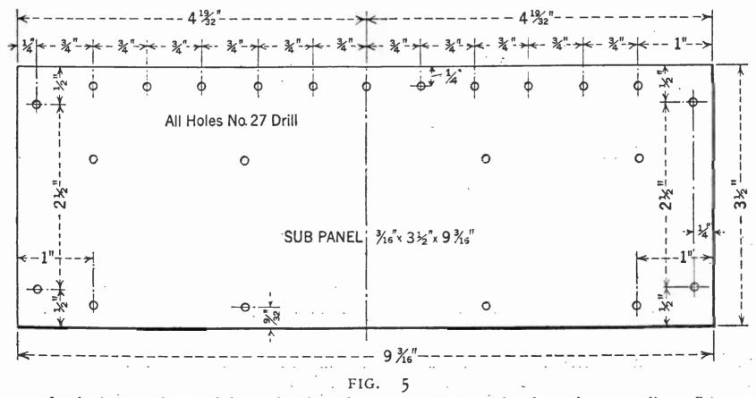
In the layout of the sub-base, the dimensions are marked starting from the center line. By actually placing the audio transformers in place, their mounting holes may be scribed
