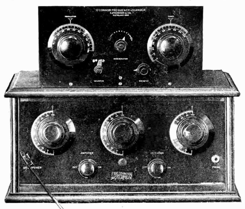
With the addition of the Frequency-Changer to any of the well-known neutrodynes, or the radio frequency receivers, the owner has an excellent six-tube superheterodyne that may be operated on a loop from medium distant stations. The receiver illustrated here is a well-known five-tube radio frequency set
