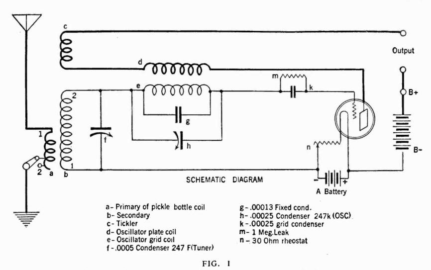
The Frequency-Changer unit that may be added to any receiver to make it into a super-heterodyne
