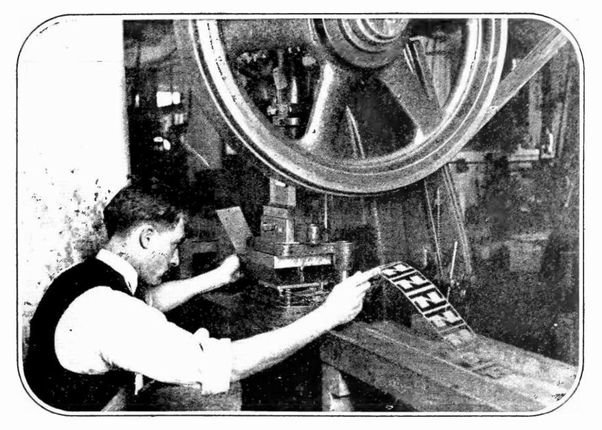
STAMPING OUT THE STEEL LAMINATIONS For audio-frequency transformers. Transformers, like all other radio parts, are made in very large quantities and special machines have been built for their manufacture
