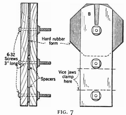
together with  $\frac{6}{32}$  machine screws 3 inches long. Place the cardboard template underneath the head of the top screw; mark and cut the slot and top as shown.
