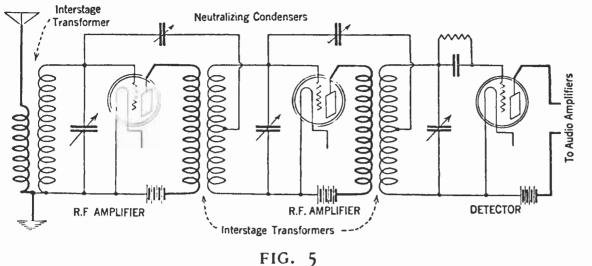
This is the conventional neutrodyne diagram of connections. Without the neutralizing condensers it would represent the connections for the first three tubes of the usual five-tube tuned radio frequency receiver
