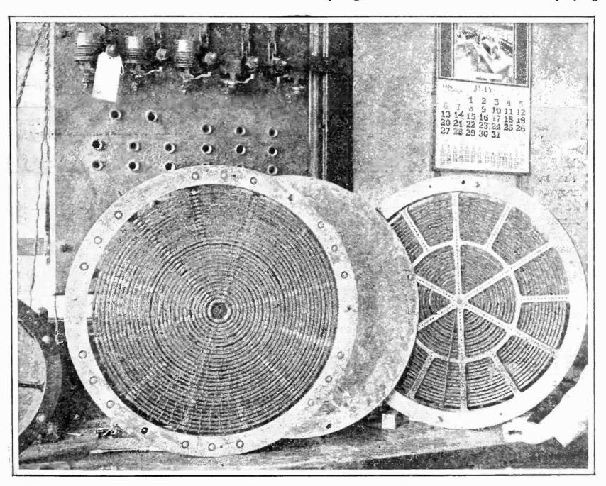
FIG. I Several of the Hewlitt Induction loud speakers in a corner of the research laboratory of the General Electric Company at Schenectady
