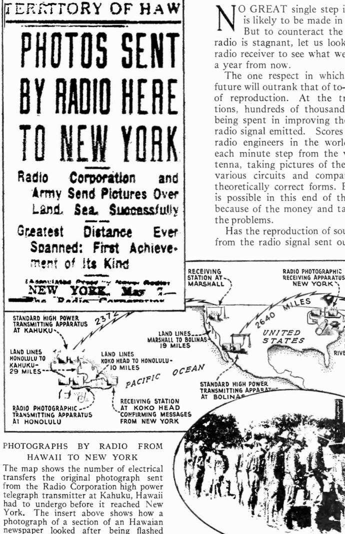
through the ether to New York. The lower insert is a radio-transmitted photo-
