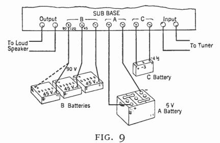
Here is how the batteries, A, B, and C are connected to the binding posts on the sub-base
