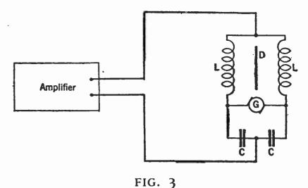
The circuit diagram of the Hewlitt induction loud speaker. L L are the two flat coils; D, the aluminum diaphragm; G, a direct current generator; and C C,
