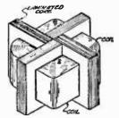
Note the quadruple core sur-rounding the coil, forming an almost perfect path for the flux within the coil. The core is a special grade of laminated sili-con steel that provides highest permeability and lowest hyster-esis loss, with consequent maxi-mum conductivity in the mag-metic circuit of the transformer. Price \$10.00. West of Rocky Mts., \$10.50.
