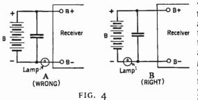
tube set having no by-pass condenser, or else a very small one, oscillations and howling often result. The effect is the same as using a B battery partly run down—it adds resistance to the circuit. Therefore put a large condenser directly across the B battery as shown in Fig. 4 B. If the lamp lights dimly when the set is
