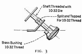
Shows the mechanical arrangement of the balancing condenser plate and mount. It is to be mounted on the sub-panel in the rear of the radio frequency secondary coil
