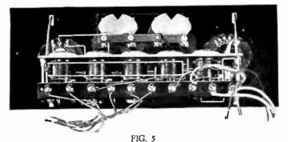
This is a rear view of the receiver shown in Fig. 8. The simplicity of the layout is brought out thoroughly from this viewpoint. It will be noted that the sockets extend far enough beneath the sub-base to allow wiring to be made at approximately the level of the socket prongs. The manner of fastening the sub-base and binding post strip to the Bruno bracket is very satisfactory The manner of fastening and very substantial
