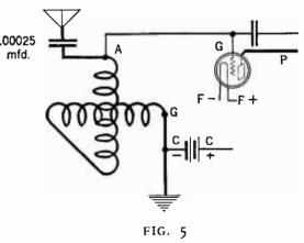
the variometer will work equally well with two or four tubes. A set in Washington, District of Columbia, using four dry cell tubes, gave good loud speaker volume on  $\kappa$ HJ. With two tubes,  $\kappa$ HJ was easily heard on head phones. I logged seventyfive stations on a loud speaker in one month.
