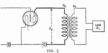
Transformers are used to "match" impedances. In the case shown here, for maximum transfer of power from tube to load,
