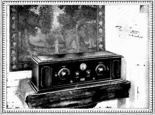
N the quest for a set that would give greater distance and selectivity and still be economical and simple in design, Frederick H. Drake and Glenn H. Browning, both doing research work at Harvard University, set to work mathematically to see just how much could be developed by a tuned radio frequency transformer.
