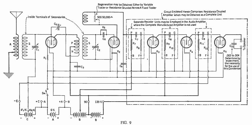
This is the circuit diagram of the RADIO BROADCAST "Aristocrat". Note that the connections of C3 have been altered. They were incorrectly shown in the diagram accompanying the constructional article on this circuit on page 30 of RADIO BROADCAST for November. A .5 mfd. condenser should be tried across the B battery, which may improve the tone. Amperite ballasts may be used for filament control in each of the tubes
