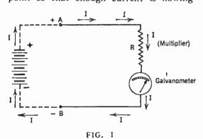
This diagram shows how a resistance and a current measuring device are employed to determine voltage
