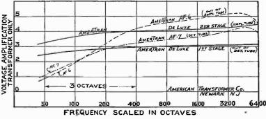
The AmerTran De Luxe is a transformer of moderate size and weight, enclosed in a strong metal case with mounting holes at both top and bottom so that it may be inverted, affording simplified connections. While the AmerTran De Luxe will improve any set, appreciation of its uniform amplifying qualities can best be realized when operated in conjunction with straight line frequency loudspeakers, such as the best cone and disc types, and with a tube in the last stage capable of handling the output.
