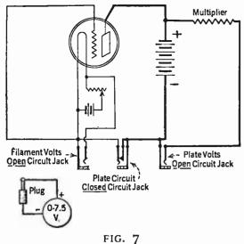
By connecting three jacks in each tube circuit, it is possible to use one meter for many different purposes. In order that several different multipliers will not be required, one multiplier may be arranged with a short-circuiting switch in the plug circuit
