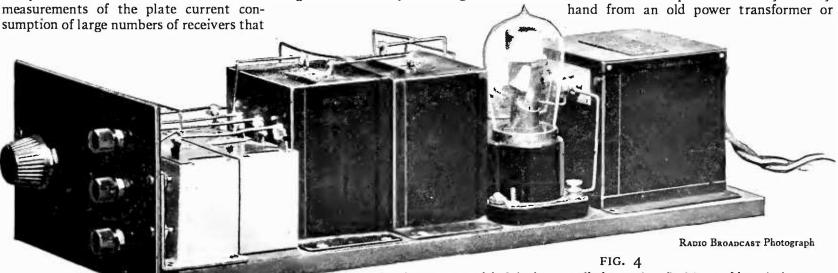
A compact model of the battery eliminator described here. Note the large condensers which are employed in the filter circuit to insure a smooth d. c. output
