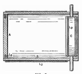
FIG. 2 Details of the winding of the radio frequency coupler. L3 is the primary; L2 the secondary, and Lp the variable tickler coil. The actual winding specifications are contained in the accompanying article sequently chosen for the receiver to be described.
