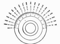
Practically even separation over half the dial with a Straight Line Frequency Condenser
