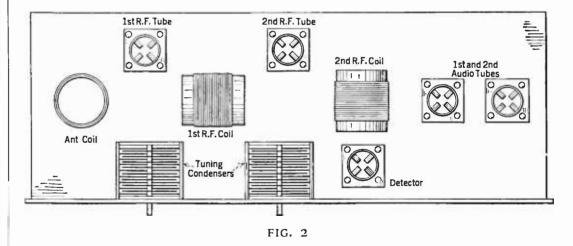
ling between the coils. This placement can be approximated by the home experimenter in his own construction. Individual test must be made to determine the point at which satisfactory neutralization is obtained in the regular manner.
