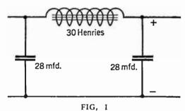
Two types of filter circuits. That shown in Fig. 1A is the "smoothing" filter popular in 1924 while the circuit, shown directly above, is the "brute force" or reservoir type so highly efficient
