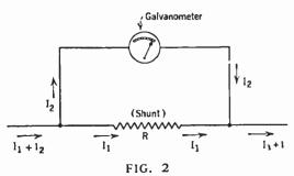
A shunt resistance is employed in order that only a small percentage of the total current in the circuit passes through the meter
