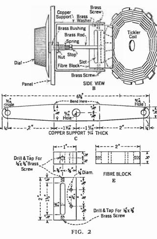
whole idea of the device rests in the use of a brass rod bent as shown in Fig. 3D, and a slotted fibre block as shown in Fig. 2 E. The slot takes up all the up-and-
