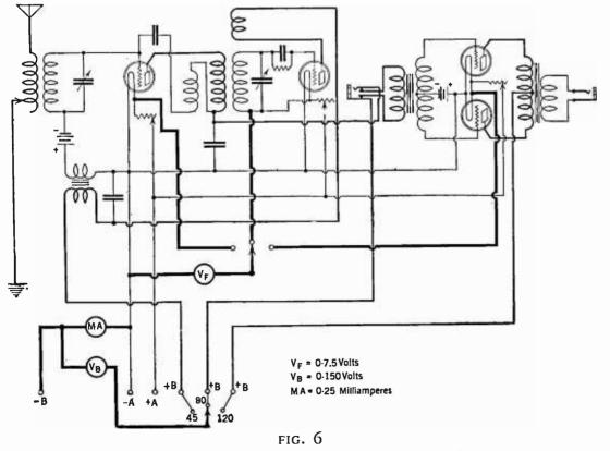
This circuit diagram shows how to connect a filament voltmeter, a plate voltmeter, and a plate milliammeter in a RADIO BROADCAST FOUR-tube Knockout receiver
