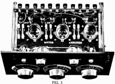
Another RADIO BROADCAST Phonograph Receiver converted into an "Aristocrat" by the use of a three-stage Muter resistance-coupled amplifier
