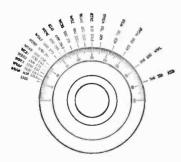
Stations partially separated and tuning slightly improved with a Straight Line Wave Length Condenser
