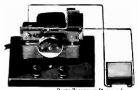
RADIO BROADCAST Photograph FIG. 2 Showing condenser connection across vibrating contacts of a battery charger
