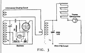
made from the several readings obtained. The circuit diagram for the layout is shown in Fig. 3. To measure the resistance of a coil, the procedure is as follows, assuming that readings are to be taken at 1500 kc. (200 meters) 1200 kc. (250 meters) 1000 kc. (300 meters) and so on, for every 50 meters up the scale to 545 kc. (550 meters.)
