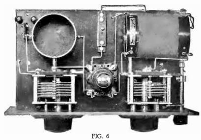
A Phonograph Receiver using the National Regenoformer Kit and the Browning-Drake circuit with a Heath resistance coupled amplifier unit. A 199 tube used in the radio frequency part of the circuit to save current and facilitate neutralization
