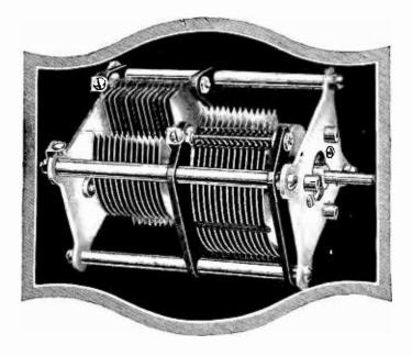
The principal objection to many Straight line Frequency condensers now on the market is that they "hog" too much panel space; thus making it necessary to re-arrange other instruments on the panel or rebuild the set entirely to allow enough room for the scythe-like sweep of the S. L. F. rotor.
