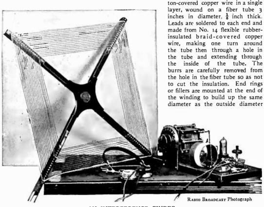
AN INTERFERENCE FINDER Of typical form. This was made in the RADIO BROADCAST Laboratory. One Duplex variable condenser tunes both loop and the R. F. secondary, which feeds into a crystal detector
