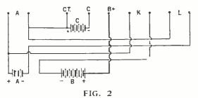
will supply it with all the necessary filament, plate, and grid voltages. The circuit diagram of the transmitter is given in Fig. 1, and the connections for battery operation are given in Fig. 2. Fig. 3 is the circuit diagram of the power unit. No changes in the transmitter itself are necessary in changing from battery operation to a.c. operation; it is merely necessary to connect the various binding posts somewhat differently so as to obtain proper operation.
