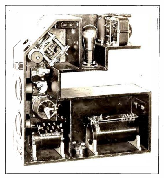
THE INTERIOR OF THE OSCILLATOR BEFORE WIRING
