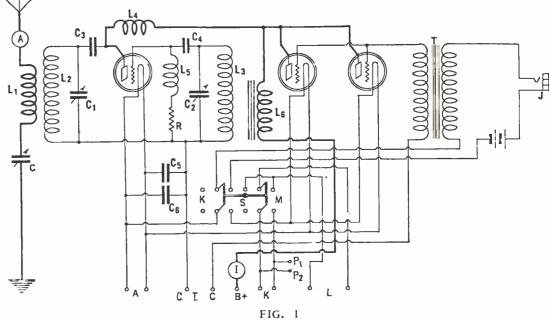
was obtained by plotting wavelength against the settings of the grid (left-hand) tuning condenser dial. In adjusting the set, the grid-circuit tuning condenser is set at the desired reading, and the plate and antenna condensers are then adjusted for maximum efficiency as indicated by the plate milliammeter and antenna ammeter.
