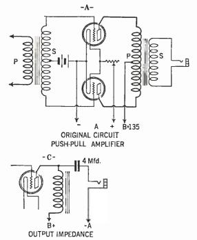
straight stage employing one of the transformers used in the reflex stage, or a new push-pull amplifier may be used utilizing special Silver-Marshall or Samson transformers. Two 112 tubes in parallel, as shown in Fig. 2, will give somewhat greater output than a single tube
