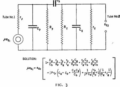
pendent on the constants of the plate circuit of the second tube. For our purpose it will be sufficiently accurate to consider rg infinite as long as the second tube is biased sufficiently. Cg may be expressed as:
