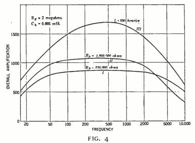
in other portions of the range. Accordingly, the frequency characteristic becomes poorer as the coupling resistance is increased.
