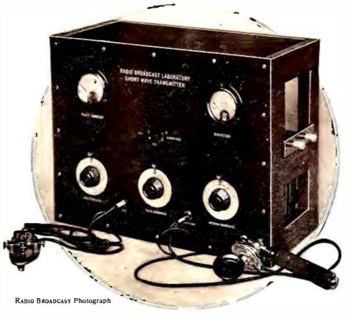
Either Battery or A. C. Operation Possible—Transmits C. W. Signals or Phone at Option
