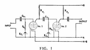
tential is applied to the grid leak resistance, Rg2, of the second tube, while the direct component is kept back by the blocking condenser Cb2. The grid of tube No. 2 is so connected that the drop in the grid leak resistance is the alternating component of grid voltage. In this stage the action is exactly like that in the preceding one.
