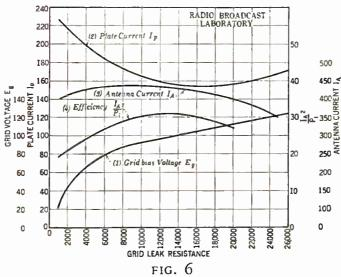
ing the coupling merely the distance between the top of the plate coil and the top of the antenna coil was measured. The curves show that there is a considerable increase in efficiency when using very loose coupling. With very close coupling and with a coupling of  $4\frac{1}{2}$  inches the antenna current is practically the same but the difference
