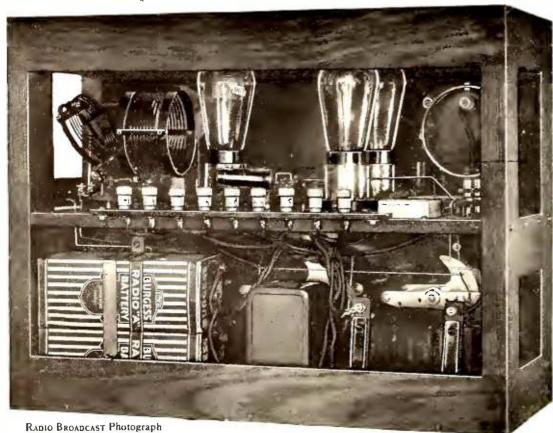
THE SHORT-WAVE TRANSMITTER As viewed from the rear. The upper and lower compartments into which the set has been divided makes possible a very compact arrangement. The Heising choke coil, modulation transformer, variable condensers, and microphone batteries, are all placed beneath the shelf
