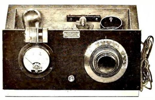
THE CRYSTAL-CONTROLLED MASTER OSCILLATOR See Fig. 2 for the circuit diagram
