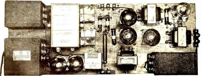
THE COMPLETE PUSH-PULL AMPLIFIER AND B SUPPLY
