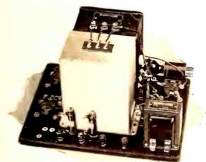
THORDARSON 210 TYPE POWER AMPLIFIER This amplifier, mounted on a special metal chassis, uses the Thordarson Power Compact R-210. Provides "A," "B," and "C" current for one UX-210 power tube and "B" voltage for the receiver. Employs one 216-B or 281 rect.fier.
