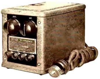
AN INEXPENSIVE B UNIT BY Modern, of Toledo. The maximum voltage output at 25 mils. is 185 volts, and at 30 mils., 175 volts. The Modern B Compact lists at \$26.50 without Raytheon tube. The voltage at the power tube tap may be reduced by inserting a fixed resistor in the fuse clips provided within the case
