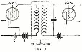
A transformer is used to connect two tubes working as radio-frequency amplifiers. The number of turns on the primary for maximum amplification is controlled by the input and output impedance of the tubes used. For a given set of tubes and at a given frequency there is a number of turns which will give maximum amplification.
