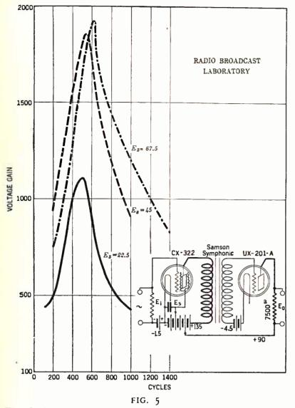
There is often some advantage in a highly peaked amplifier. These curves were made with a Samson "Symphonic" transformer when used with a screened-grid tube
