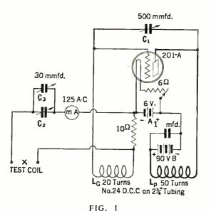
A setup developed for matching coils
