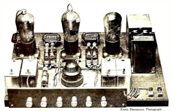
USING 222 TYPE TUBES IN AN AUDIO AMPLIFIER This is the conventional resistance-coupled amplifier using two screened-grid tubes and one 171 power tube. The little cap on top of the tube is the signal grid connection. The values of resistance, etc., are given on Fig. 5
