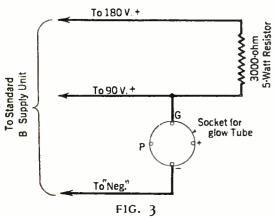
How to add a glow tube to any B supply device. The addition of the glow tube will increase the stability and all-around efficiency of the circuit.
