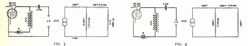
be large. The equivalent circuit is shown in Fig. 3. Here is a source of voltage, a series impedance representing the plate resistance of the tube, a shunt impedance representing the choke, and a series impedance representing the condenser, and another impedance representing the loud speaker. The shunt impedance is a bypass for the audio frequencies and naturally must be large compared to the remainder of the circuit, *i.e.*, the series impedance of the loud speaker and the condenser.
