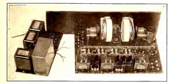
POWER UNIT AND RECEIVER PROPER In the event that the power unit is to be mounted elsewhere than right beside the receiver, the front panel for the latter may be smaller
