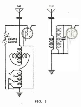
winding. The voltage is obtained by tapping the secondary winding at a predetermined point.
