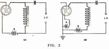
shows the result, 32 per cent. of the current which should flow through the loud speaker being lost. The condenser which is in series with the loud speaker must take its share of the voice currents which are circulating in this circuit, and for that reason its impedance, compared to that of the loud speaker, must be small.
