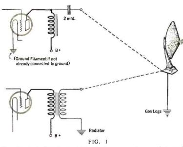
Showing how a single lead to the set, plus a ground connection, can be used with either transformer or choke coil output device to operate a loud speaker at some distance from the receiver
