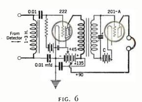
lf still greater discrimination against unwanted audio signals is desired, this manner of connecting the detector to the audio stage might be useful. The low-impedance choke in the input short circuits the low frequencies. The bypass condenser across the audio transformer secondary shunts out the higher audio tones and leaves only a narrow band around 1000 cycles
