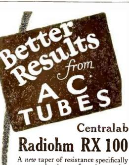
to control volume of receivers using the new AC tubes. A variable resistance in R. F. plate circuit or R. F. filament circuit, customarily used in battery circuits, cannot be used with AC tubes without destroying the delicate balance of voltage for efficient operation.
