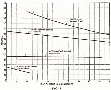
producing power units with good regulation is important. As a result several methods are at present in vogue whereby power units can be constructed with comparatively good regulation. The use of a glow tube in the output circuit of a power unit will cause the regulation of the unit to be excellent over the entire range of useful load. A group of curves taken on a power unit utilizing a glow tube are given in Fig. 5. Also it has been found that by
