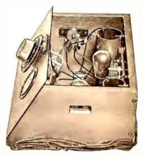
THE AUXILIARY OSCILLATOR AND DETECTOR The circuit diagram of this unit is shown in Fig. 3
