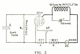
The master oscillator circuit with quartz crystal control
