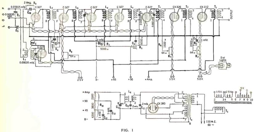
The circuit diagram of the 45-kc. a.c. super-heterodyne
