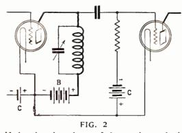
If the plate impedance of the previous tube is very high the entire input coil of the following tube may be used to approach the maximum amplification possible. This is true when the screened-grid tube is used, for its plate impedance is very high indeed, of the order of one half to one megohm
