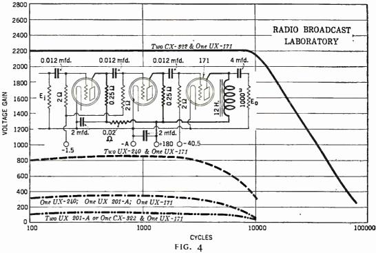
When the total a.c. voltage appearing in the plate circuit of the last tube is divided by the input voltage to the first tube, this kind of curve results. In each case the final tube was a 171, and various combinations of high-mu tubes, screened grid tubes, and standard 201-A tubes were measured and the results plotted as shown
