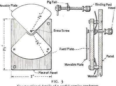
Constructional details of a useful vernier condenser
