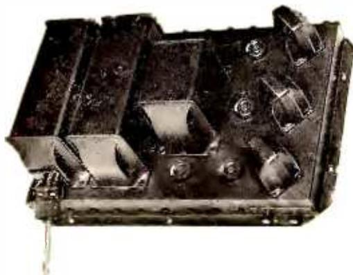
PAC 2 requires one 227 for first stage, two 210 tubes for last stage, one UX 281 and one UX 874 tube. Price, without tubes, \$175.00
