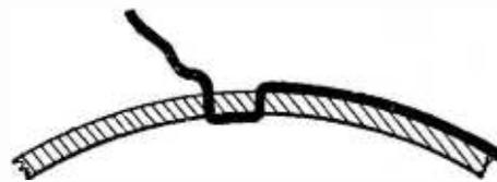
Fig. 4—Securing the end of the wire
