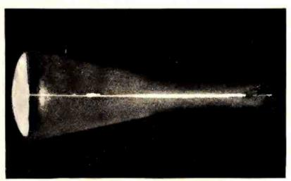
Fig. 3—The Braun cathode-ray tube photographed in a dark room.
