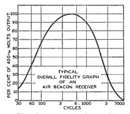
The above curve indicates the overall fidelity of the average airbeacon receiver.
