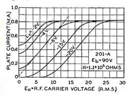
The curves on this sheet are for a 201A-type tuhe operated with a resistance load in the plate circuit from a battery potential of 90 volts. Five curves are shown for grid biases from —2 to —20 volts. These curves were made by measuring the plate current as the r.f. input voltage was gradually increased from 0 up to 30 volts. The plate currents obtained with the various input voltages were then plotted and the series of curves shown on this sheet was obtained
