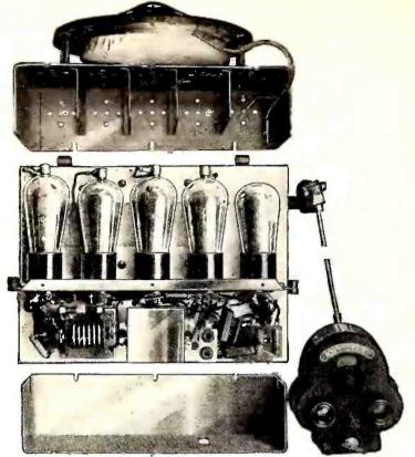
An "exploded" view of the Bosch automobile radio chassis.
