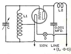
Fig. 4-A variation of Fig. 1 with parallel feed.
