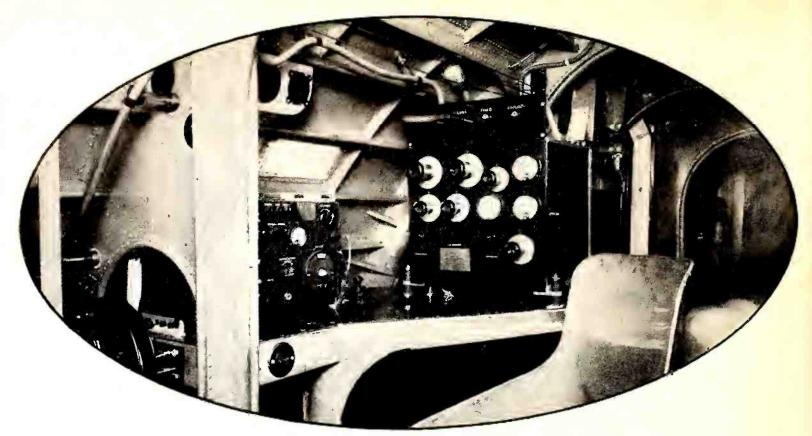
View of radio transmitting and receiving apparatus in a modern Navy airplane.
