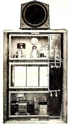
Rear view of audio-frequency voltmeter.
