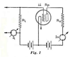
three times the tube resistance, three times as much voltage will appear across the load as across the tube (we are speaking of a.c. voltages), and therefore the voltage amplification will be mu × 75 per cent.
