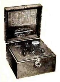
One of the new test oscillators for the radio service laboratory is now ready. It will deliver a modulated radio-frequency voltage at any point in the broadcast band (500 to 1500 kilocycles) and at 175 and 180 kilocycles. The tuning control is calibrated with an accuracy of 2 per cent.
