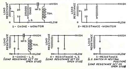
Fig. 2—Circuits obtainable with loading device.
