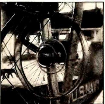
View of a wind-driven motor generator.
