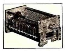
America, Micalex insulation is employed. Typc R-39 insulation, a special development of the Radio Frequency Laboratories, can be supplied if desired in place of Micalex. The condensers are of variable capacities from 0.0005 to 0.00005 mmfd. Prices range from \$47.50 down to \$41.00
