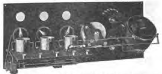
Interior view of Fada Receiver, Detector and Two Stage Amplifier
