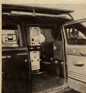
Included in cross-country demonstration unit is the GPL Utility Projector, with "3-2" intermittent which permits use with I.O. camera for film telecasting from remotes.
